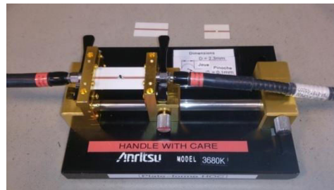
Fig. IV-8. Picture of the TRL measurement platform with the calibration standards.
