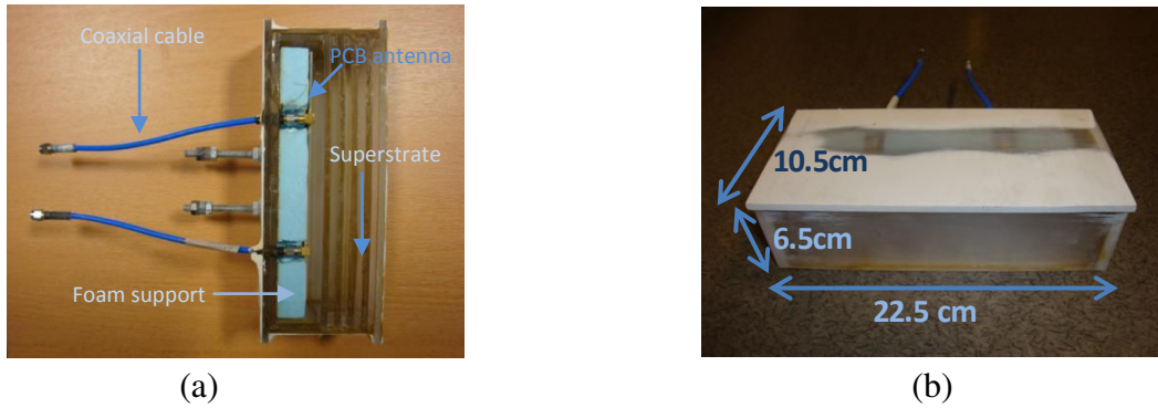
Fig. III-19. Final patch antenna array with superstrate: (a) top view and (b) perspective view of the closed box.
