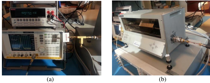
Fig. IV-15. Zoom of the measurement setup: (a) DC load and Bias Tee, (b) diode PCB with two quarter-wavelength microstrip lines
