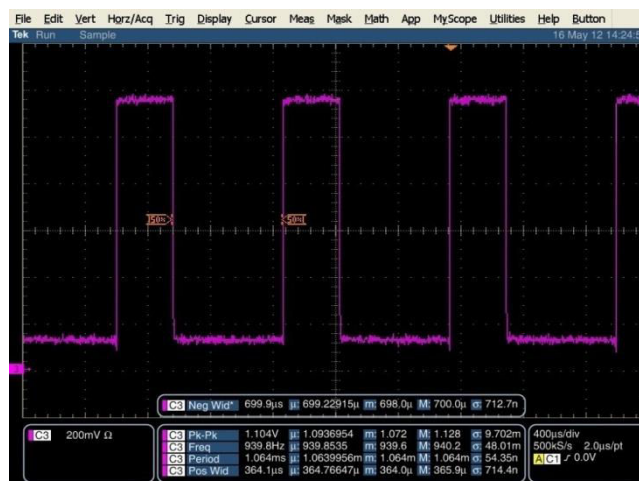
Fig. II-24. Oscilloscope print screen of the SB_out output during a successive AM signal receiving.
