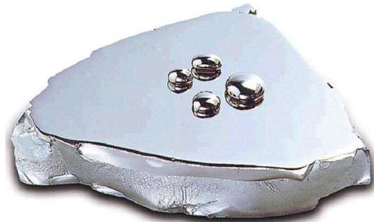
FIGURE 1.2: A sample of Zr-based metallic glass [2].
