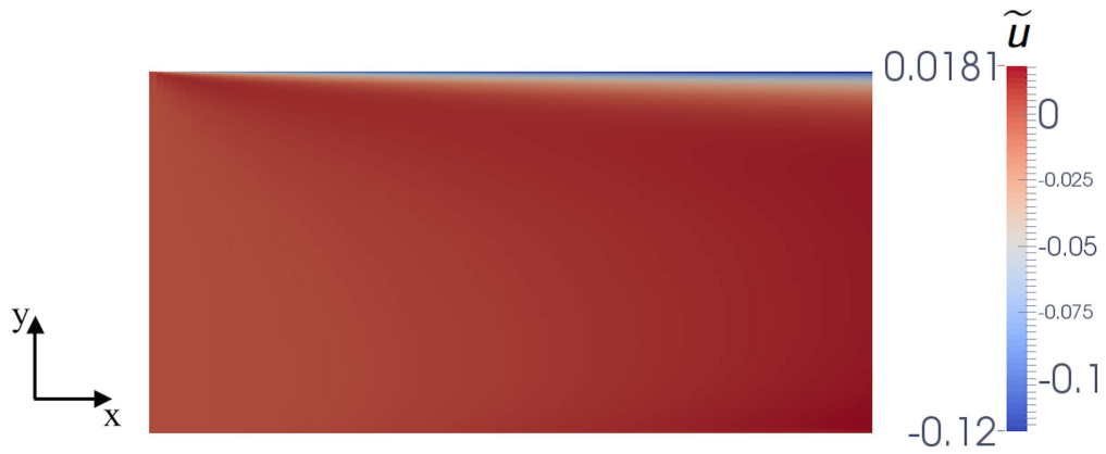
Figure 3.32: Perturbation \tilde{u} of the x component of the gas velocity at the first stage of the drying process obtained with w_{in} = 10 \text{ m.s}^{-1} and with the mesh 100 \times 283 .
