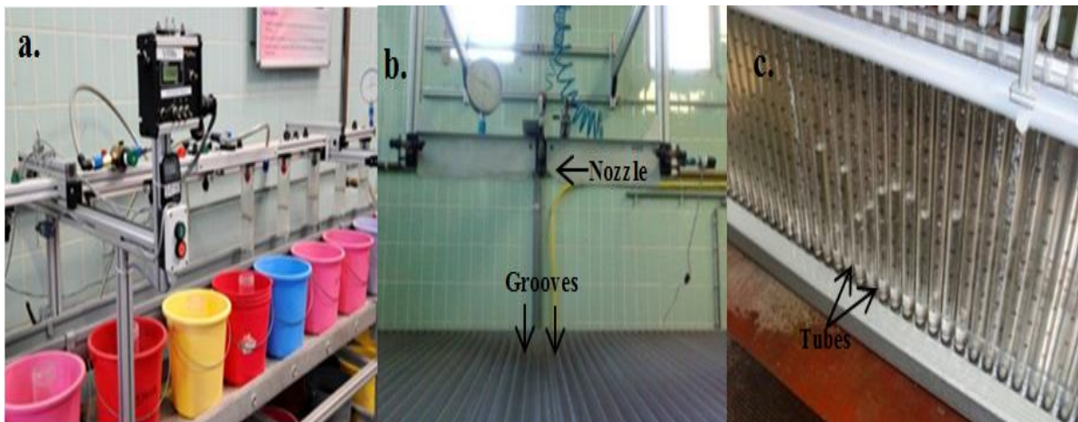
Figure 7.4. Non-imaging techniques for spray characterization at ILVO's Spray Tech Lab: (a) flow rate test bench and (b) & (c) horizontal patterner
