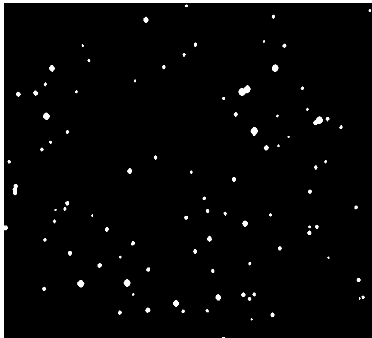
Figure 6.18. Spray droplet image shown in Figure 6.15. after applying morphological operations
