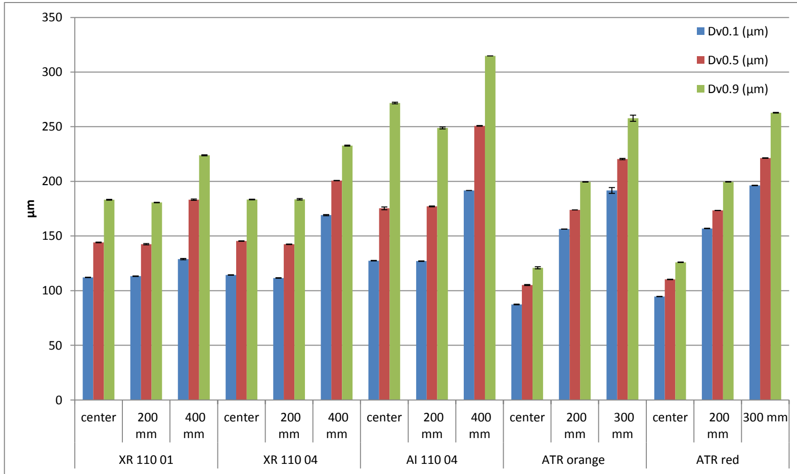
Figure 6.24. Droplet size distribution parameters D_{v0.1} , D_{v0.5} and D_{v0.9} ( \mu\text{m} , mean \pm std.) for five nozzle pressure combinations (Table 6.3) at 0.5 m below the nozzle at three measurement points (center, 200mm, edge of the spray)
