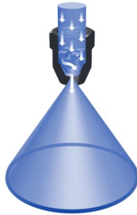
Figure 2.5. Liquid sheet and droplet formation from a hollow cone nozzle ( www.lechler.de )
