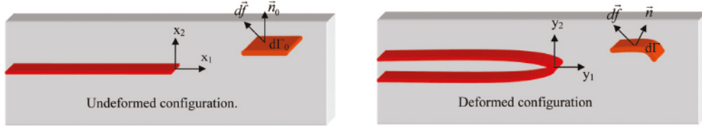
Figure 5.23: Undeformed and deformed geometries of the strip specimen. We define the first Piola Kirchhoff stress ( \mathbf{S} ) and the true stress ( \mathbf{T} ). With \vec{df} , the force acting on a material surface of area d\Gamma_0 in the undeformed configuration with a unit normal vector \vec{n}_0 . After deformation, d\Gamma_0 becomes d\Gamma with new unit normal vector \vec{n} . The first Piola Kirchhoff stress tensor \mathbf{S} is defined by \vec{df} = \mathbf{S}\vec{n}_0 d\Gamma_0 . The true (Cauchy) stress tensor \mathbf{T} is defined by \vec{df} = \mathbf{T}\vec{n} d\Gamma .
