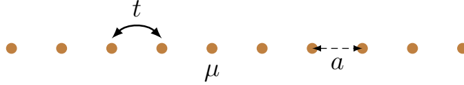
Figure 3.1: One-dimensional tight-binding lattice. \mu is each site chemical potential, a is the lattice constant and t is the nearest neighbor hopping amplitude.
