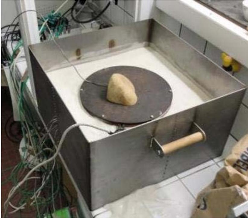
Figure 5.1: Experimental hearth. The sand is fully saturated with water.
