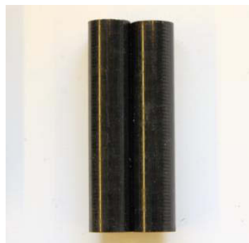
Figure 2.9 Example of specimen used in the testing of surface energy: two cylinders are glued along a generatrix
