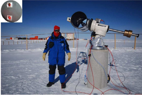
Fig. 1. The PML instrument at Dome C, Antarctica in January 2011. The top-left insert shows the subapertures mask of PML.
