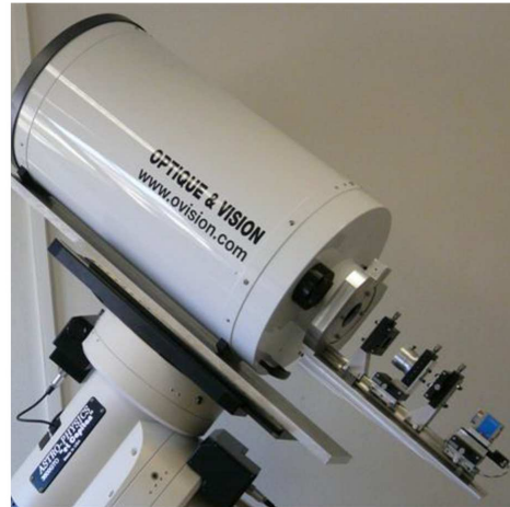
Figure 2. The PML instrument backside with the collimating and imaging lens, the Dove prism and the CCD camera.
