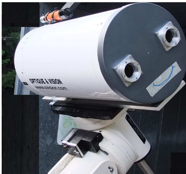
Fig. 1. The PML/PBL mask configuration on the telescope entrance pupil.
