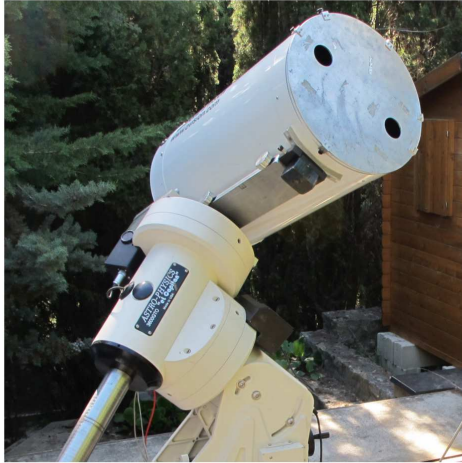
Figure 1. PML telescope front side with the implemented two sub-apertures mask. Pupils diameter D = 6\text{cm} , baseline B = 26.7\text{cm} .
