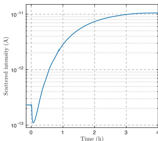
Figure 4.6: The growth of graphene on Ni(111) can be followed by monitoring the first order diffraction peak while dosing ethene ( $\text{C}_2\text{H}_4$ ). Here the time  $t = 0$  on the abscissa corresponds to starting the dosing of ethene. First nickel carbide forms and the intensity drops. As soon as this converts to graphene the intensity increases since graphene exhibits a larger corrugation than Ni(111). The whole growth process continuous over several hours.
