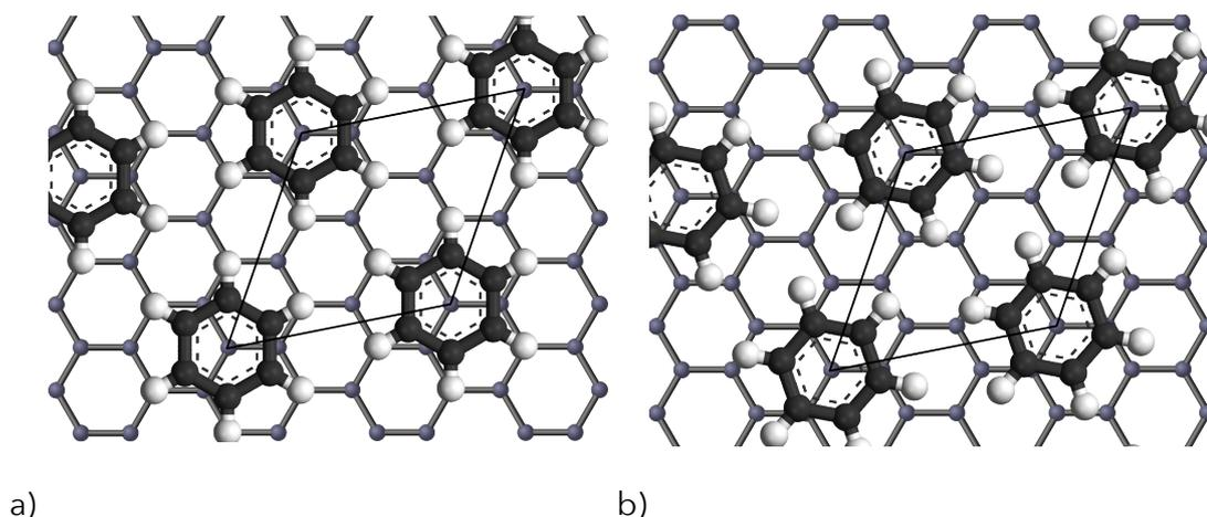
Figure 6.4: Illustrations of the commensurate  $(\sqrt{7} \times \sqrt{7})\mathbf{R}19^\circ$  structure. a) The hydrogen atoms are positioned on top of first layer carbon atoms. b) The hydrogen atoms are turned away from the carbon atom positions. This orientation agrees with our recent MD calculations [136].
