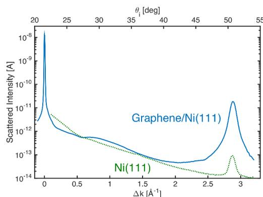
Figure 4.5: Comparison of the scattered intensities for graphene/Ni(111) and clean Ni(111) versus  $\Delta k$ . Both scans were taken along the  $\overline{\Gamma M}$  direction with the crystal at room temperature and a beam energy of 8 meV. The intensity of the diffraction peak is increased on the graphene covered surface which indicates a larger corrugation of the surface electron density compared to the pristine Ni surface.
