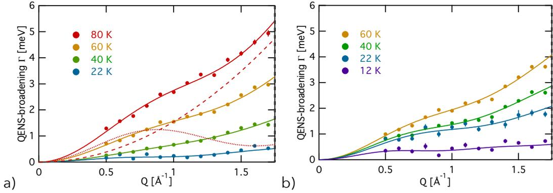
Figure 8.6: The quasi-elastic line broadening  $\Gamma$  as a function of momentum transfer,  $Q$ , for a range of sample temperatures. The error bars are too small to be visible for most data points. The continuous lines show the results from fitting Eq. (8.2) to the broadening. Both contributions to the broadening have been shown separately for the 80 K data: the dashed red line shows the contribution from collisional diffusion and the dotted red line show the contribution from jump diffusion.
