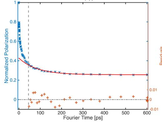
Figure 5.8: Normalized polarization versus Fourier time  $t$  at  $\Delta k = 0.38 \text{ \AA}^{-1}$  in  $\overline{\Gamma M}$  direction. Blue crosses: ISF of 0.06 ML  $\text{H}_2\text{O}$  on the graphene surface at 125 K. Red line: single exponential decay fitted to the experimental data. Orange crosses: Residuals. Grey dashed line: lower threshold at 45 ps.
