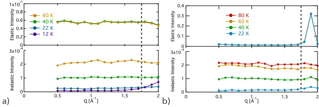
Figure 8.4: Elastic and inelastic intensities as a function of momentum transfer,  $Q$  at different temperatures. Values to the right of the dashed grey line have not been taken into account for analysis of the quasi-elastic broadening. a) Results for the D-96-7 substrate. b) Results for the Papyex substrate.
