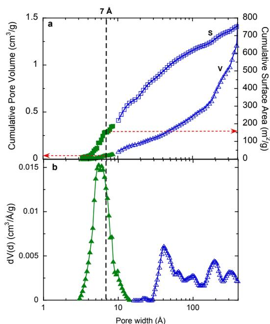
Figure 9.3: a) Cumulative pore size distribution (triangles) and surface area (squares) and b) incremental pore size distribution of the carbon aerogel obtained from the 77 K  $N_2$  (blue open symbols) and room temperature  $CO_2$  (green closed symbols) adsorption measurements derived by QSDFT ( $N_2$ ) and NLDFT ( $CO_2$ ) models, respectively, with slit/cylinder geometry. Arrows indicate the pore volume,  $V$ , and surface area,  $S$ , of pores with pore width  $w < 7 \text{ \AA}$ .
