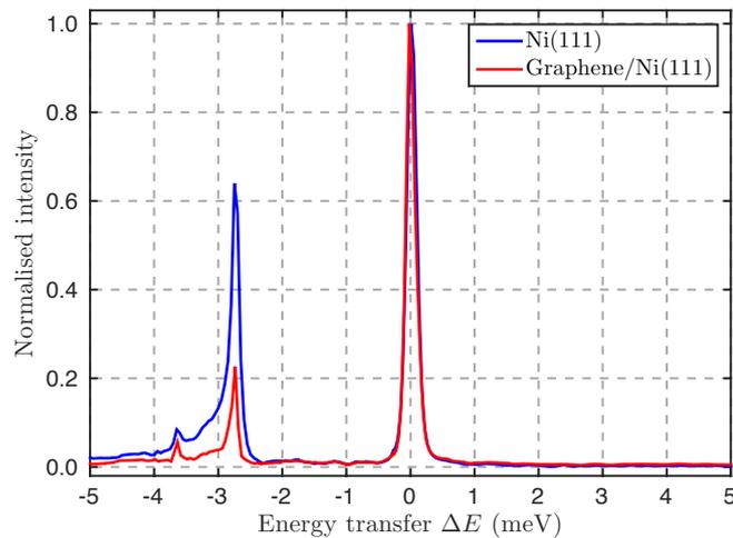
Figure 4.8: Comparison of the phonon spectra for graphene/Ni(111) and Ni(111). The spectrum was taken along the  $\bar{\Gamma}\bar{M}$  azimuth at an incident angle  $\theta_i = 18.2^\circ$ ,  $E_i = 8$  meV and the sample was cooled down to 150 K. Despite the diffuse elastic peak at 0 energy transfer both the Rayleigh mode at -2.7 meV and the longitudinal resonance at -3.6 meV can clearly be seen. The intensity of the Rayleigh mode is smaller on the graphene covered surface.
