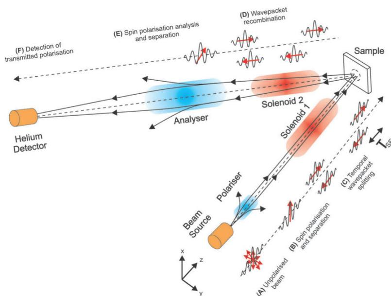
Figure 3.13: Schematic drawing of the HeSE instrument at the Cavendish Laboratory. Explanations of the different parts are given in the text. From [48].
