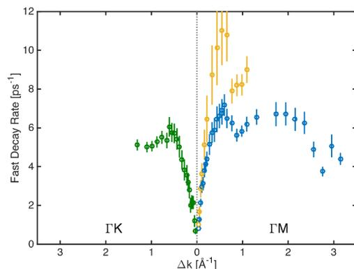
Figure 5.16: Fast decay rate  $\alpha_{fa}(\Delta k)$  of 0.06 ML H<sub>2</sub>O on graphene versus  $\Delta k$ . Blue and green: temperature 125 K; yellow: temperature 110 K.
