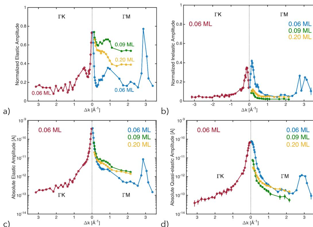
Figure 5.9: Quasi-elastic and elastic amplitudes of different H<sub>2</sub>O coverages at 125 K versus  $\Delta k$ . a) and c) relative and absolute elastic polarization amplitudes  $I_{el}(\Delta k)$  and  $\tilde{I}_{el}(\Delta k)$ , respectively; b) and d) relative and absolute quasi-elastic polarization amplitudes  $I_{qe}(\Delta k)$  and  $\tilde{I}_{qe}(\Delta k)$ , respectively.
