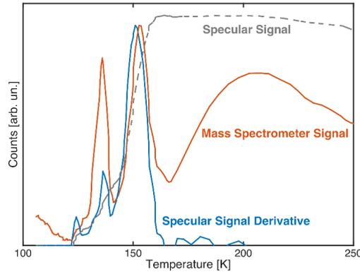
Figure 5.5: Mass spectrometer signal and derivative of the specular helium signal  $dI/dT$  versus temperature  $T$  during thermal desorption of water from graphene/Ni(111), dosed at 100 K. The applied heating rate in the range 130 - 180 K was  $\beta = 0.11$  K/s. Orange solid line: mass spectrometer signal. Blue solid line: derivative of specular signal  $dI/dT$ . Grey dashed line: specular signal.
