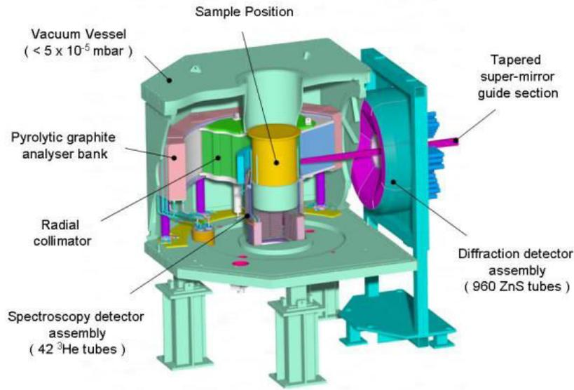
Figure 3.6: Schematic drawing of the instrument OSIRIS at ISIS. From [22]
