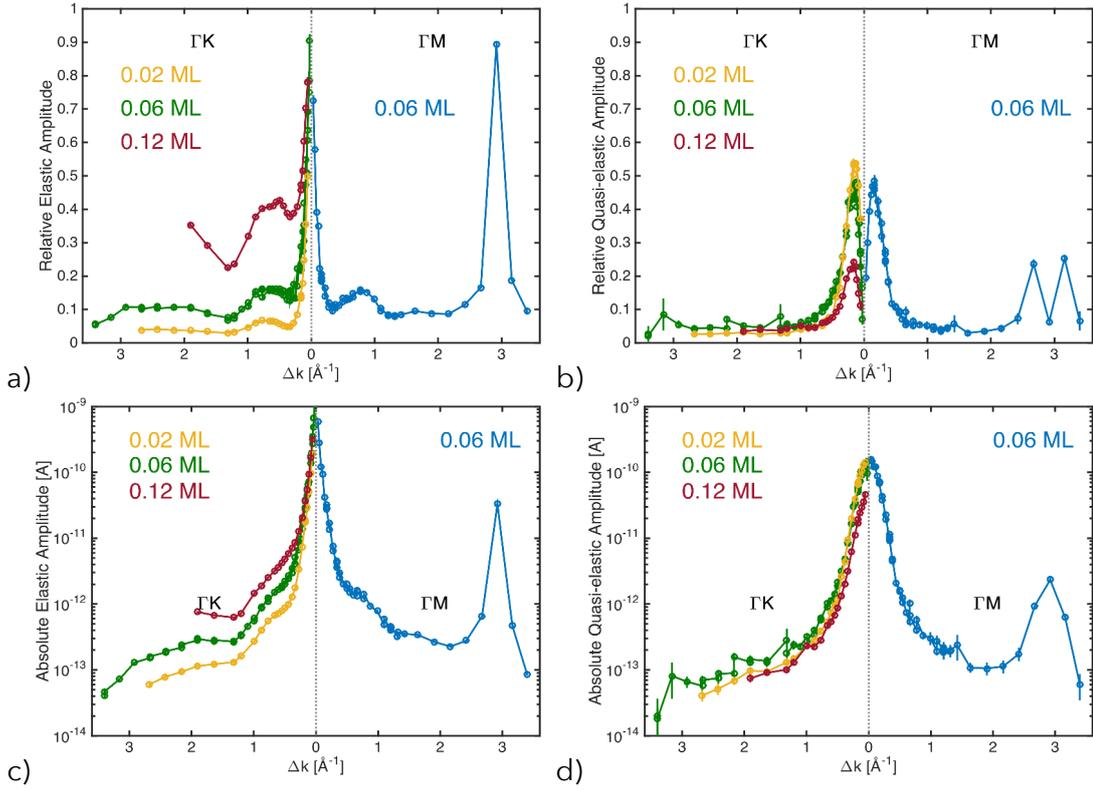
Figure 7.7: Quasi-elastic and elastic amplitudes of different surface coverages of benzene at 110 K. a) and c) Normalized and absolute elastic polarization amplitudes,  $I_{el}(\Delta k)$  and  $\tilde{I}_{el}(\Delta k)$ , respectively b) and d) Normalized and absolute quasi-elastic polarization amplitudes,  $I_{qe}(\Delta k)$  and  $\tilde{I}_{qe}(\Delta k)$ , respectively.
