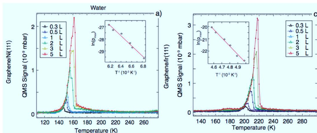
Figure 5.1: Thermal desorption spectroscopy of H<sub>2</sub>O adsorbed on the surfaces of graphene/Ni(111) and of graphene/Li(111). From [55].
