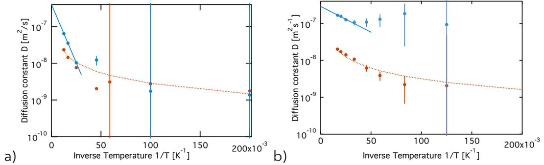
Figure 8.8: Arrhenius plots of the logarithm of the diffusion constant  $D$  versus inverse temperature. Blue dots: Experimental jump diffusion constant; blue line: Linear Fit to high temperature data; orange dots: Experimental Brownian-type diffusion constant; orange line: Theoretical Brownian-type diffusion of combined surface and collisional friction. a) Results for Papyex substrate. b) Results for D-96-7 substrate.
