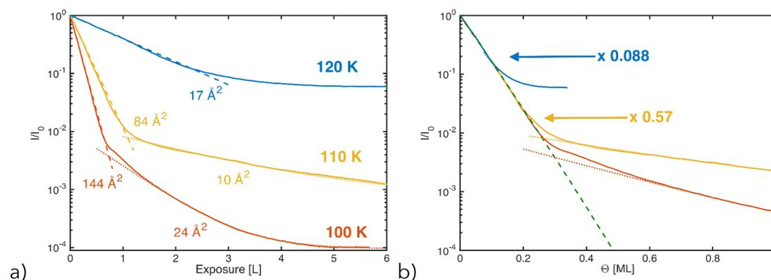
Figure 5.3: Normalized specular helium signal  $I/I_0$  versus exposure for the adsorption of H<sub>2</sub>O onto the GR/Ni(111) surface at three temperatures 100 K, 110 K, and 120 K.  $I/I_0$  is shown on a logarithmic scale. Dashed lines indicate the initial signal attenuation with the corresponding helium scattering cross section  $\Sigma_1$ . Dotted lines show an exponential fit to the helium signal at higher coverage, where a lower helium scattering cross section  $\Sigma_2$  is found.
