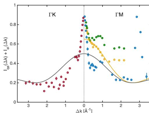
Figure 5.18: Sum of slow quasi-elastic amplitude  $I_{qe}(\Delta k)$  and elastic amplitude  $I_{el}(\Delta k)$  versus  $\Delta k$ . Blue and red: 0.06 ML coverage; green: 0.09 ML coverage; yellow: 0.20 ML coverage. Grey and yellow lines: zeroth order Bessel function  $j_0^2(\Delta k \cdot R)$  with an arbitrary amplitude plus an offset of 0.2 to match the experimental data.
