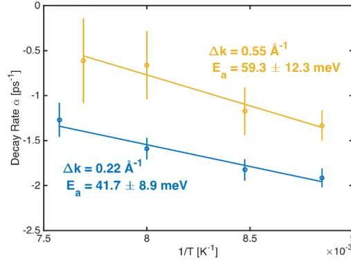
Figure 5.13: Arrhenius plot of  $\alpha(\Delta k)$  versus inverse surface temperature of 0.06 ML  $\text{H}_2\text{O}$  on graphene at  $\Delta k = 0.22 \text{ \AA}^{-1}$  and  $\Delta k = 0.55 \text{ \AA}^{-1}$ . The straight solid lines indicate fits to an Arrhenius-type model function.
