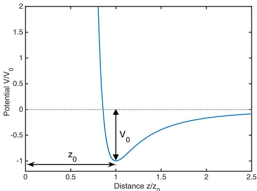
Figure 3.2: Illustration of the Lennard-Jones potential for the description of a physisorption process.  $V_0$  denotes the potential minimum,  $z_0$  denotes the distance of the adsorbate to the surface at minimum interaction potential.
