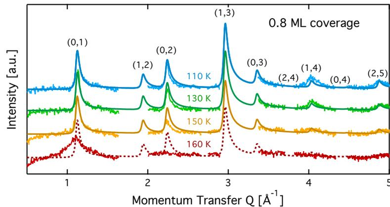
Figure 6.3: Diffraction patterns for varying temperatures at a coverage of 0.8 ML. The calculated diffraction pattern for a commensurate  $(\sqrt{7} \times \sqrt{7}) \mathbf{R}19^\circ$  monolayer is shown by the (dotted) line.
