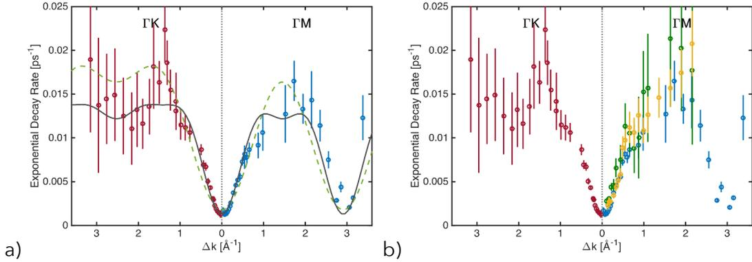
Figure 5.11: Corrected exponential decay rate of H<sub>2</sub>O on graphene at 125 K versus  $\Delta k$ . Blue and red: 0.06 ML coverage; green: 0.09 ML coverage; yellow: 0.20 ML coverage. a) Black solid line: CE model with possible jumps to the three closest sites. Green dashed line: CE model with jumps to only neighbouring sites; b) Comparison of decay rates at different surface coverages.
