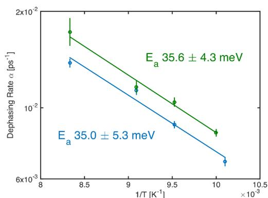
Figure 7.6: Arrhenius plot of the decay rate as a function of inverse temperature. Depicted in blue are data measured at  $\Delta k = 0.17 \text{ \AA}^{-1}$ ; depicted in green are data measured at  $\Delta k = 0.33 \text{ \AA}^{-1}$
