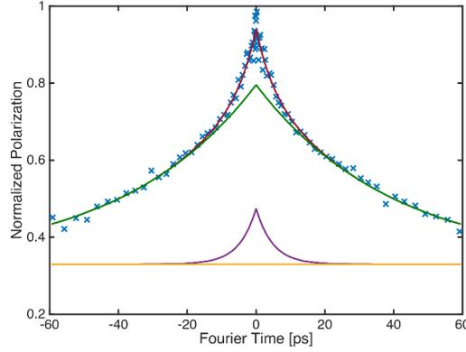
Figure 7.10: ISF at 110 K and  $\theta = 0.06$  ML,  $\Delta k = 0.17 \text{ \AA}^{-1}$ , direction  $\overline{\Gamma M}$ . The measured data are indicated by blue crosses. Yellow line: elastic contribution; green line: sum of elastic contribution and slow quasi-elastic contribution; Purple line: sum of elastic and fast quasi-elastic contribution; red line: sum of all three contributions.
