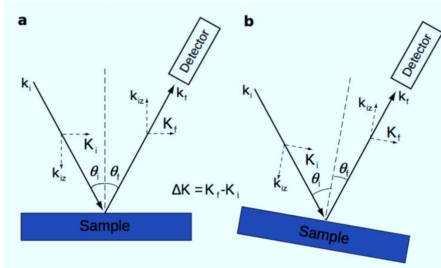
Figure 3.14: Scattering geometry at the HeSE spectrometer for specular scattering (a) and off-specular scattering (b). The total scattering angle is fixed at  $44.4^\circ$  and momentum transfer is achieved by tilting the scattering plane. From [50].
