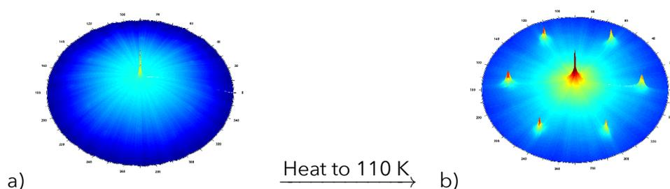
Figure 5.7: Helium diffraction patterns of water adsorbed on a graphene/Ni(111) surface. a) When dosed at 100 K,  $\text{H}_2\text{O}$  forms amorphous ice on the graphene surface; all diffraction signal is lost. b) When heated to 105 K, the original graphene diffraction pattern is recovered (pattern shown was measured at 110 K), showing only the first order (110) diffraction peak and its equivalents in the hexagonal symmetry.
