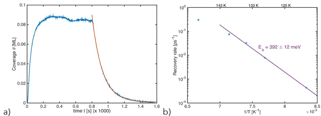
Figure 7.2: a) Exponential decay of surface coverage at 130 K after benzene exposure is stopped at  $t = 800$  s. b) Arrhenius plot of exponential decay rate (errorbars are barely visible). The point at 150 K seems to deviate from the activated behaviour and has been excluded from the fitting.
