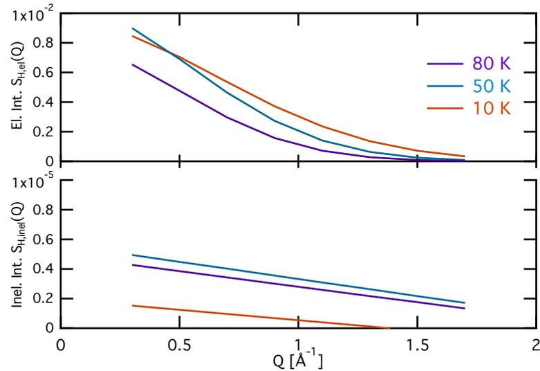
Figure 9.8: Elastic and inelastic intensities as a function of momentum transfer,  $Q$ . The data were obtained for a hydrogen coverage of the equivalent of 0.25 – 0.5 ML on CG (Tab. 9.1).
