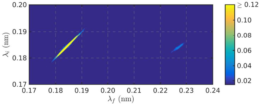
Figure 4.7: 2D wavelength intensity matrix for graphene/Ni(111) along  $\overline{\Gamma\text{M}}$  recorded at  $\theta_i = 18.2^\circ$ , a beam energy of 8 meV and a sample temperature of 150 K. The plot shows the measured probability for detecting a scattered He atom with wavelength  $\lambda_f$  versus the incoming wavelength  $\lambda_i$ . The only two visible features are the elastic peak (at  $\lambda_f = \lambda_i$ ) and the Rayleigh mode on the creation side (at larger  $\lambda_f$ ).
