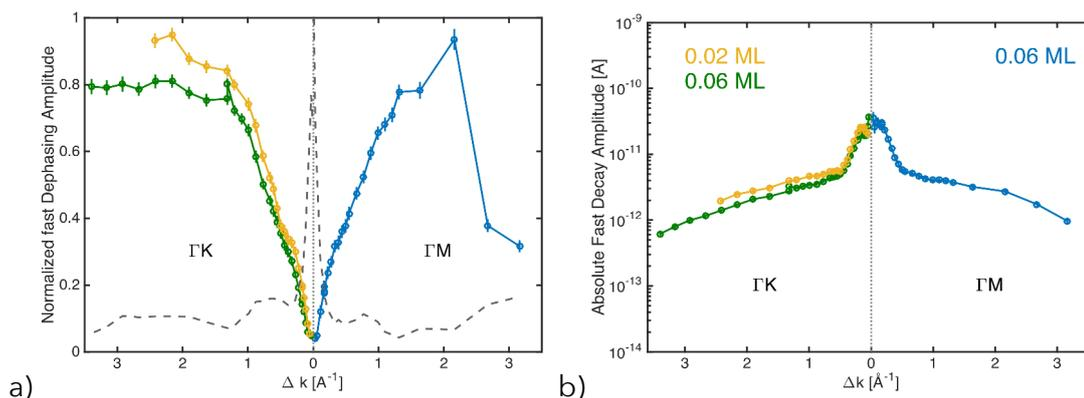
Figure 7.12: Amplitudes of the fast quasi-elastic contribution at 110 K. a) Relative amplitude  $I_{f_{qe}}(\Delta k)$ , grey dashed line: relative elastic contribution at 0.06 ML. b) Absolute amplitude  $\tilde{I}_{f_{qe}}(\Delta k)$ .
