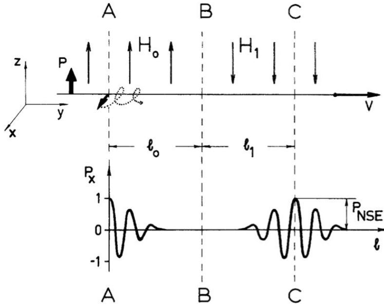
Figure 3.7: Basic illustration of dephasing of the neutron spin through Larmor precession and spin echo from [23]. A precession field  $H_0$  between A and B causes dephasing. After passing through an inverse but equal precession field  $H_1$ , a spin echo is obtained around point C.
