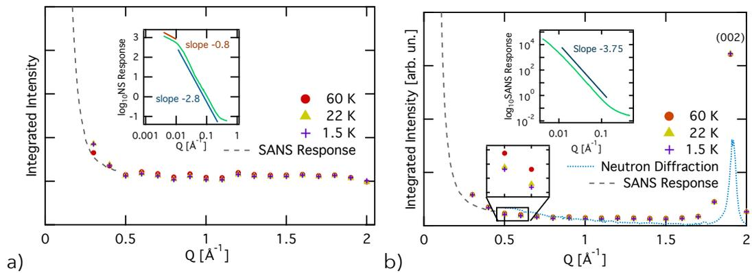
Figure 8.2: Energy-integrated intensities  $S(Q)$  obtained at IN6 for D-96-7 and Papyex after hydrogen adsorption at 1.5 K (crosses), 22 K (triangles) and 60 K (circles). The data are compared to SANS measurements (solid and dashed lines) and to neutron diffraction measurements (dotted line). a) D-96-7 b) Papyex. The (002) Bragg reflection at  $1.87 \text{ \AA}^{-1}$  is clearly visible for the Papyex sample. Insets: log-log plot of SANS response.
