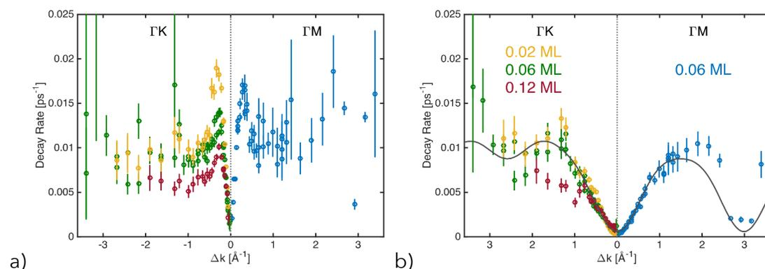
Figure 7.8: Decay rates versus  $\Delta k$  of different benzene surface coverages at 110 K. a) Coherent decay rate  $\alpha(\Delta k)$ . b) Incoherent decay rate  $\alpha_{inc}(\Delta k)$ . Grey solid line: CE model of jump diffusion.
