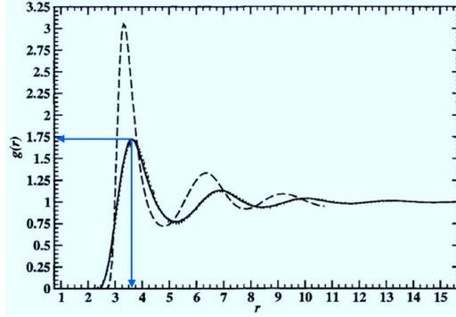
Figure 8.7: Radial distribution function  $g(r)$  of liquid para-hydrogen versus distance  $r$ , calculated by path integral simulations, from [221] (Solid line). Blue arrows: values for  $g(d)$  and  $d$  of the first maximum, which we used to calculate the collisional friction. The dashed line is of no importance for this work.
