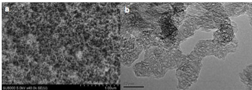
Figure 9.1: SEM a) and TEM b) image of the CG used in the experiment.
