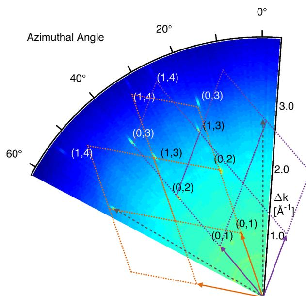
Figure 7.4: Polar colour-plot of helium diffraction signal from monolayer benzene on the surface of graphene/Ni(111) at 110 K with  $\Delta k$  along the radial coordinate and the azimuthal angle along the angular coordinate. Grey dashed arrows: Unit cell vectors of the reciprocal graphene lattice. Orange and purple arrows: Unit cell vectors of the reciprocal  $(\sqrt{7} \times \sqrt{7})\mathbf{R}19^\circ$  benzene overstructure, with selected repetitions indicated by dotted lines.
