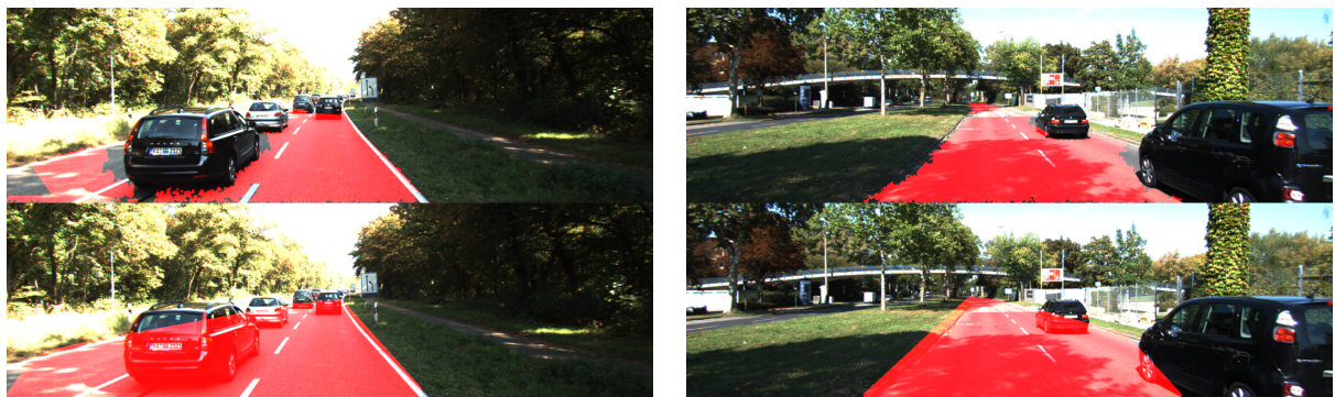
(a) Example of recovered road surface from drivable area (b) Recovered traffic area by taking convex hull operation on free road surface
