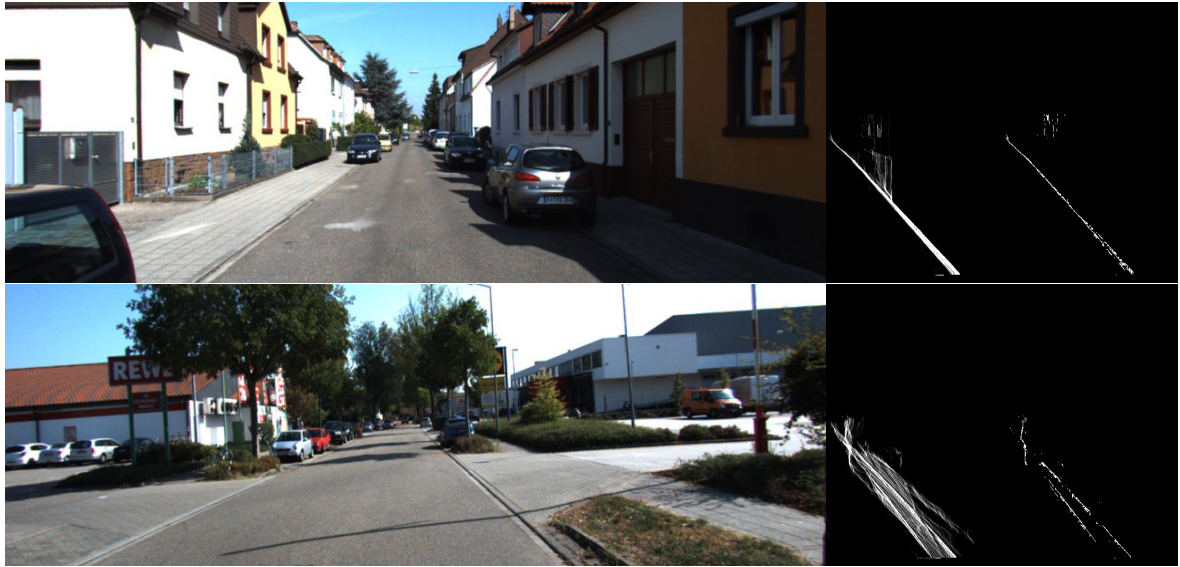
Figure 1.8 – Examples of the different V-disparity images. First row and second row show the V-disparity images from a planar road and a non-planar road respectively. Right to the original images, the first column of the V-disparity images are obtained from the entire disparity map after sky removal; the second column of the V-disparity images are obtained from the disparities on road area
