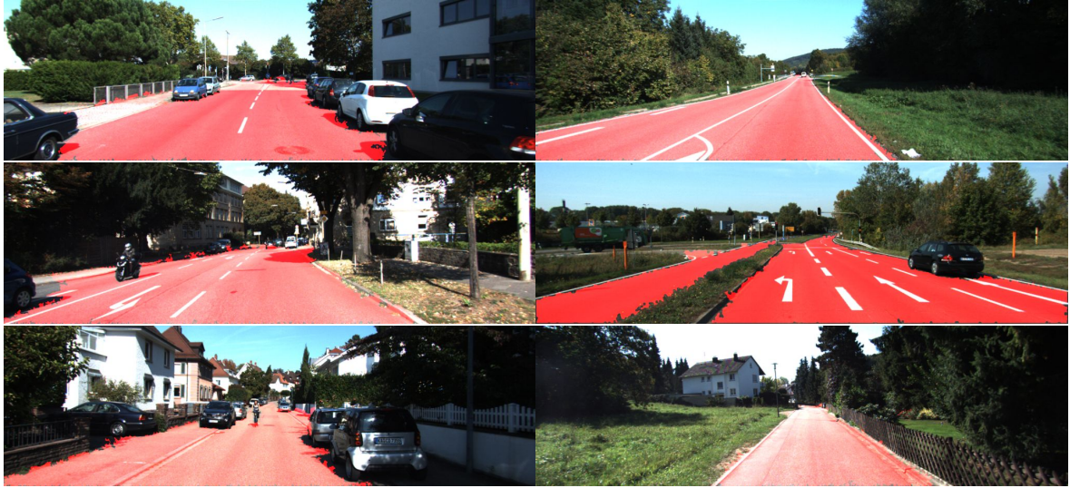
Figure 1.9 – Binary map detection results on the KITTI-ROAD dataset. Each line shows two images from different categories (see Section 1.6.1) separately.
