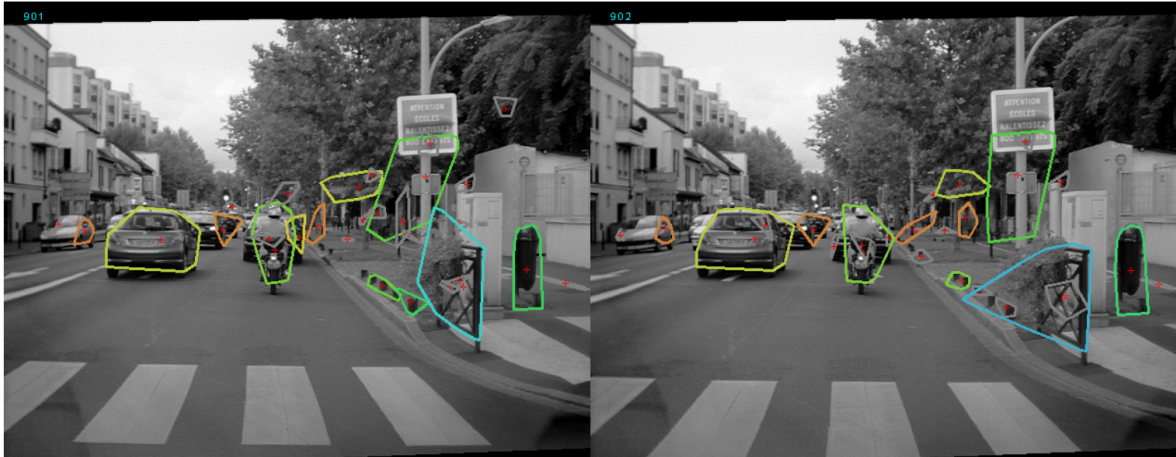
Figure 3.4 – Example of obstacle detection using all the patches in the disparity map [KB12]
