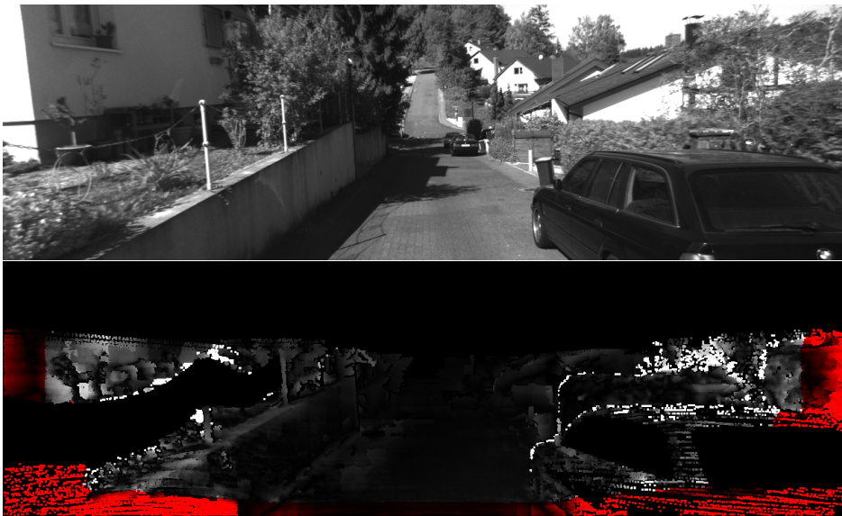
Figure 2.20 – Example of optical flow evaluation on KITTI dataset. The top image is the original image for optical flow estimation, the bottom one is the error map scales linearly between 0 (black) and \geq 5 (white) pixels error. Red in the error map denotes all occluded pixels, falling outside the image boundaries. The method of this example is presented in [YMU14]
