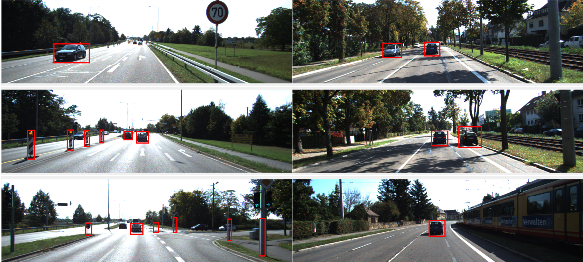
Figure 3.10 – Obstacle detection results with stereo vision in different scenarios: left column highway, right column urban road
