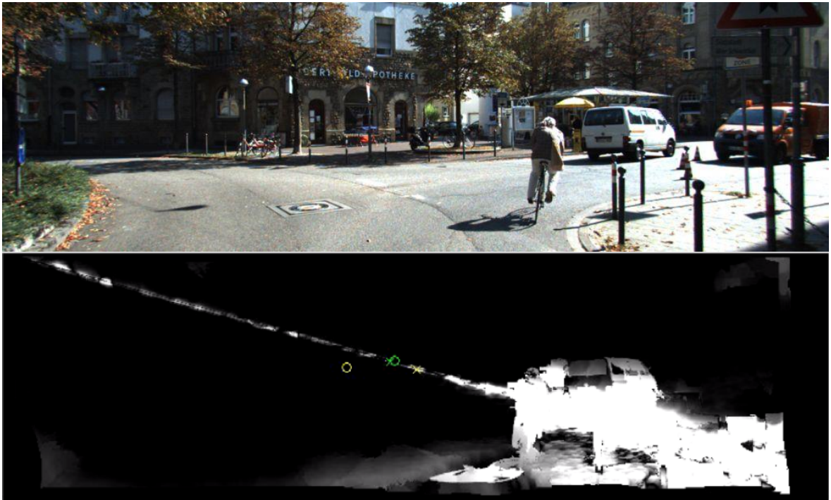
Figure 2.5 – Example of unstable detection result caused by unmodified projective depth calculation. Top: original image. Bottom: moving pixels detected by Eq.2.8
