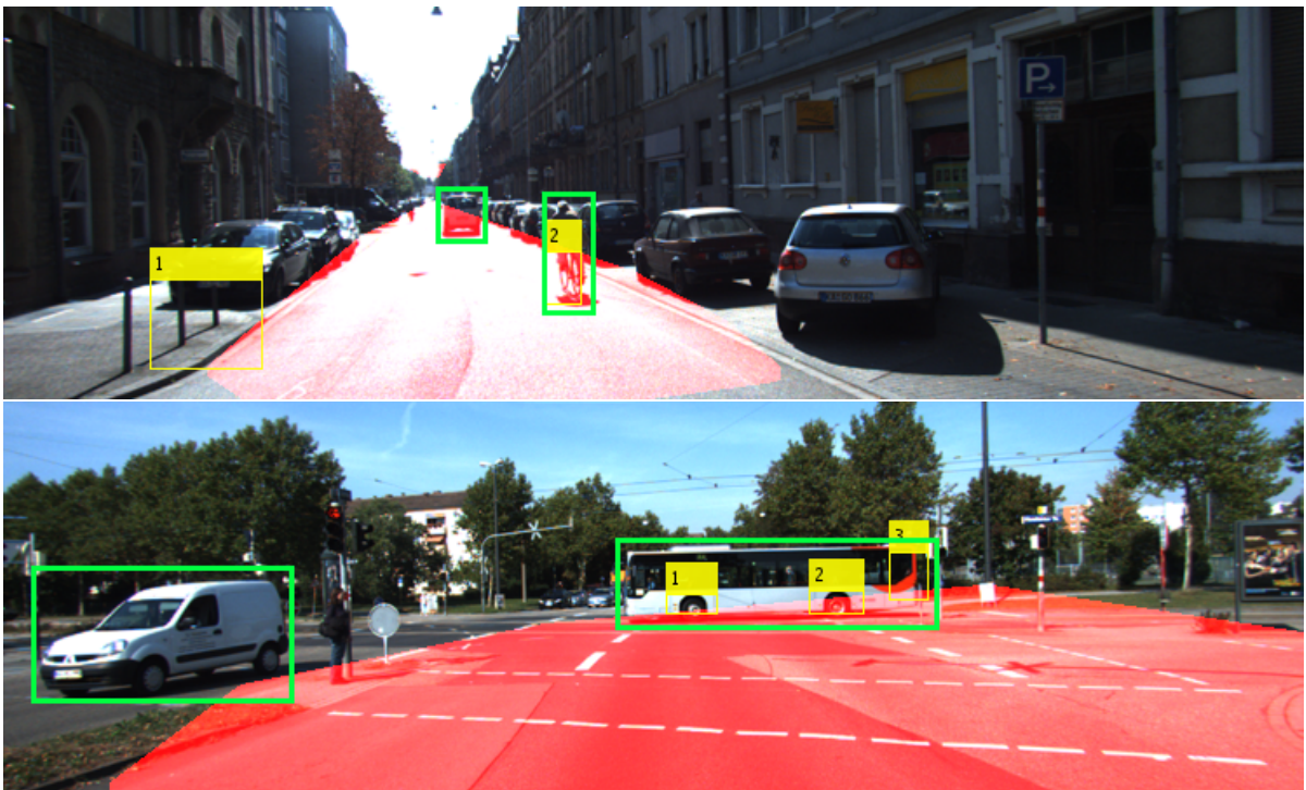
Figure 2.18 – Example of detection result of Dataset 1 and Dataset 3, red area are the ROIs, yellow boxes are the detection result, green boxes are the ground truth
