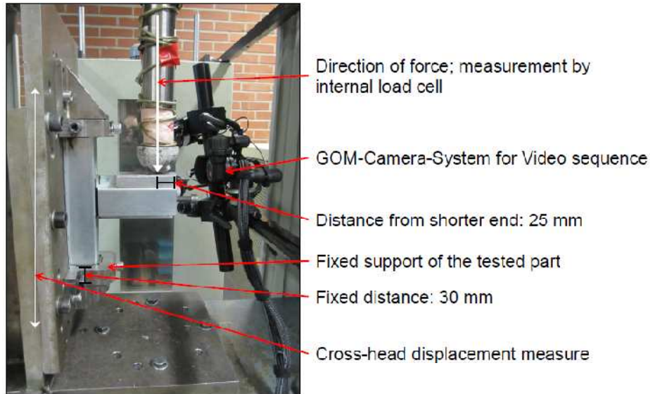
Figure 5-5. T-joint test setup under longitudinal loading
