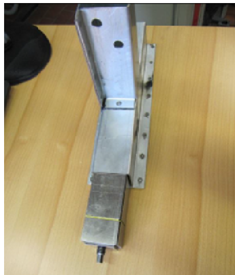
Figure 5-4. Stiffness block placed inside the horizontal beam
