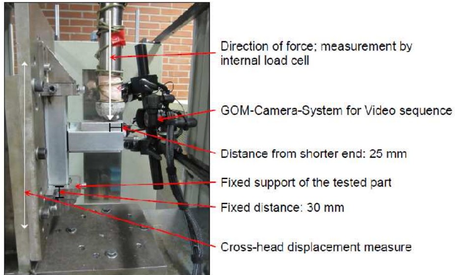
Figure 5-5. T-joint test setup under longitudinal loading
