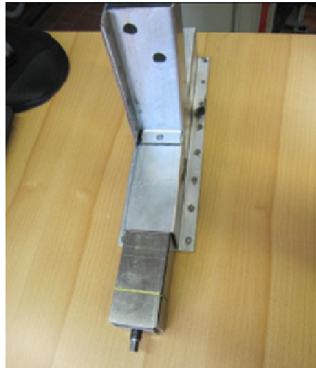
Figure 5-4. Stiffness block placed inside the horizontal beam
