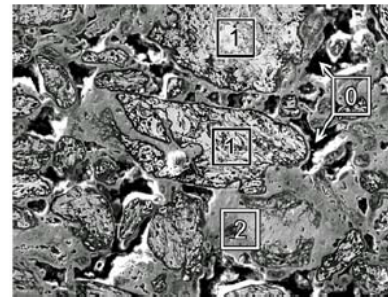
Fig. 10 SEM micrograph of polished surface of CoAlO/Co-Al cermet.
