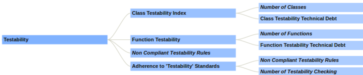
Figure 9.2: Computation of testability in SquORE’s ISO9126 OO quality model.
