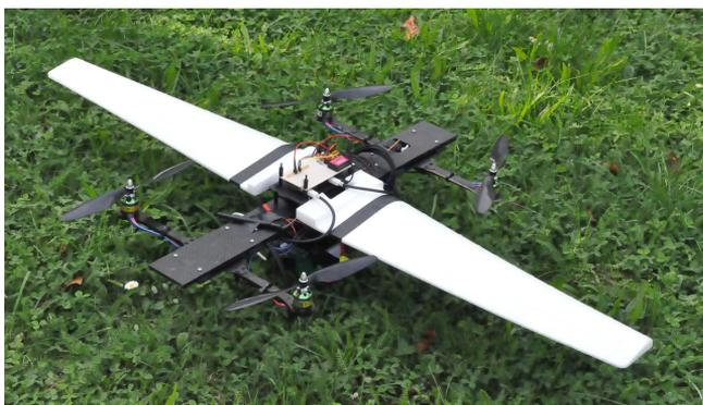
**Figure 3:** Quad-plane experimental platform.
