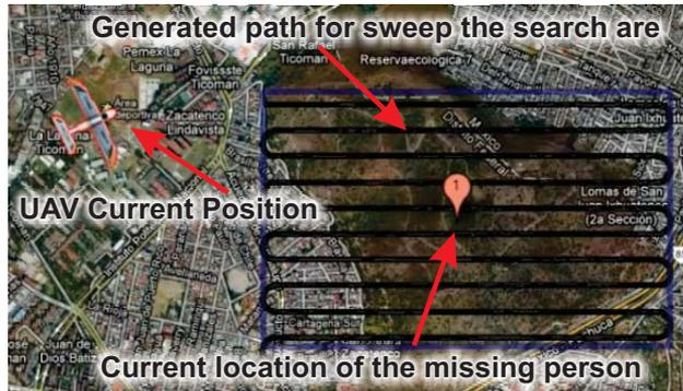
Figure 3.9: The path generated to weep the search area.
