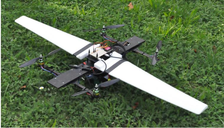
**Figure 8.6:** Experimental platform: The Quad-plane Convertible MAV equipped with imaging, inertial and altitude sensing systems.
