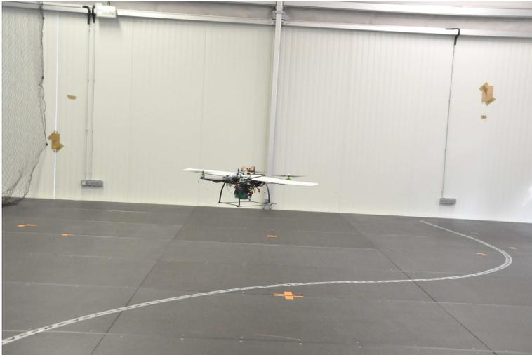
**Figure 8.20:** Road-following mission: The rotorcraft flying in the experimental area during real-time tests.
