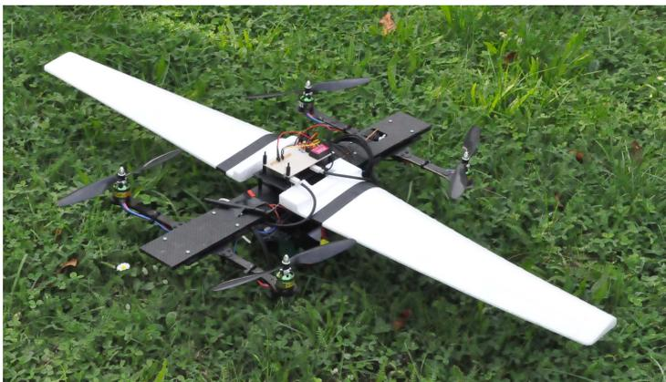
**Figure 4.4:** Quad-plane experimental platform, developed at HEUDIASYC laboratory.
