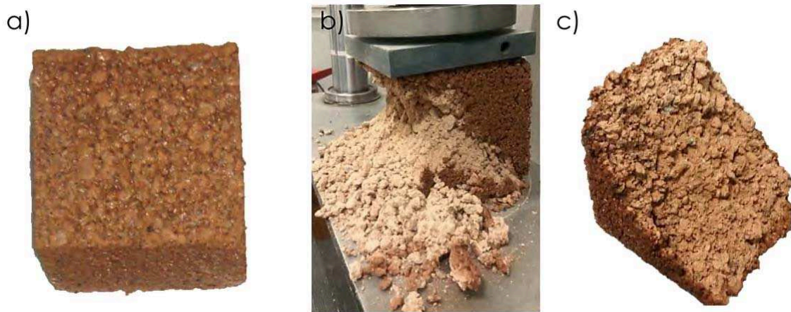
Figure 25. a) Geopolymer dry concrete cubes; b) during c) and after breaking.
