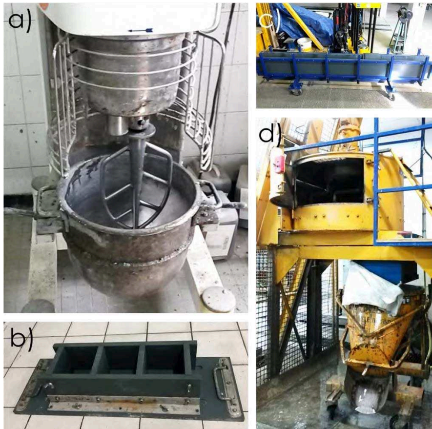
Figure 6. a) 10 L mixer, d) 200 L mixer, b) 100 x 100 x 100 mm cubes and c) 3000 x 280 x 150 mm prism mould used to cast geopolymer concretes.
