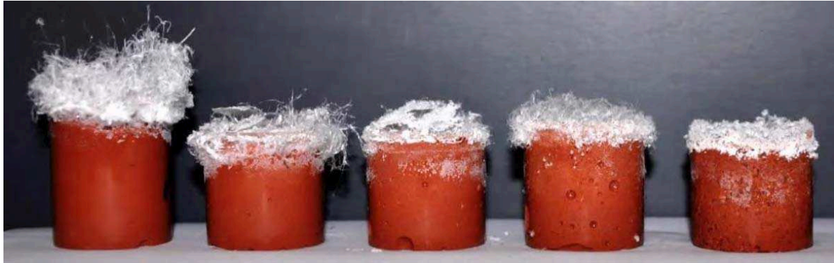
Figure 36. Efflorescence observations on GP14.5 geopolymer having from left to right: 0%, 40%, 50%, 60% and 70% of sand by mass at 7 days.
