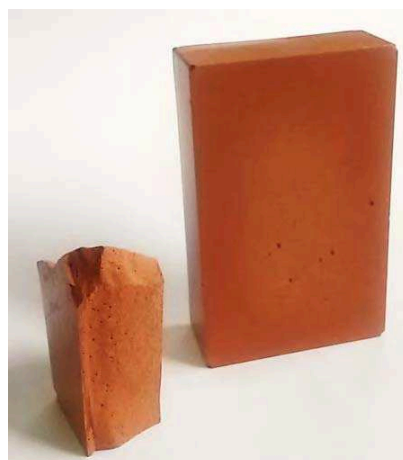
Figure 26. Metakaolin-based geopolymer prism and piece of prism after breaking (GP14.5).
