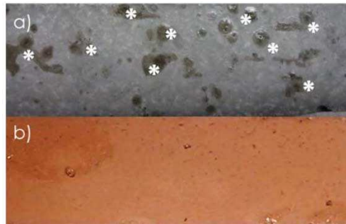
Figure 25. Surfaces, at 100 days, of 2x2x2cm OPC (a) and GP (b) mortar made with 10% of opal and 90% of marble, cured at 20°C and 95% R.H..
