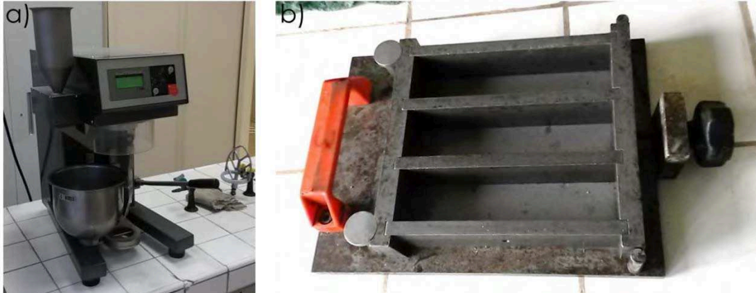
Figure 12. 5L mixer a) and b) 4 \times 4 \times 16 cm moulds used to cast geopolymer mortar.
