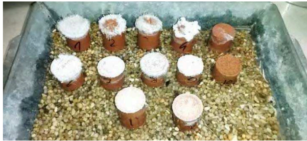
Figure 10. Capillary rise test on geopolymer cylinder showing efflorescence.
