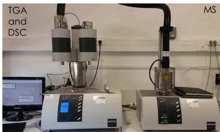
Figure 13. NETZSCH STA 449F3 TGA and DSC (left) and NETZSCH QMS 403C (right).
