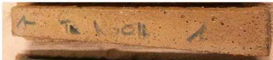
Figure 23. 2x2x16cm geopolymer mortar made with the alluvial sand with opal (sand e) cured at 60°C immersed in a 1M NaOH solution for 28 days.
