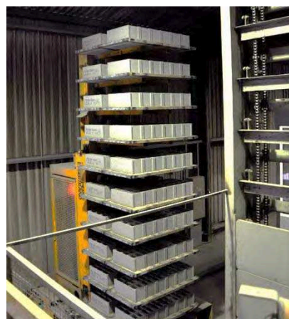
Figure 11. Automatic conveyor in SEAC “Guiraud frères” precast plant, 09120 Varilhes, France.
