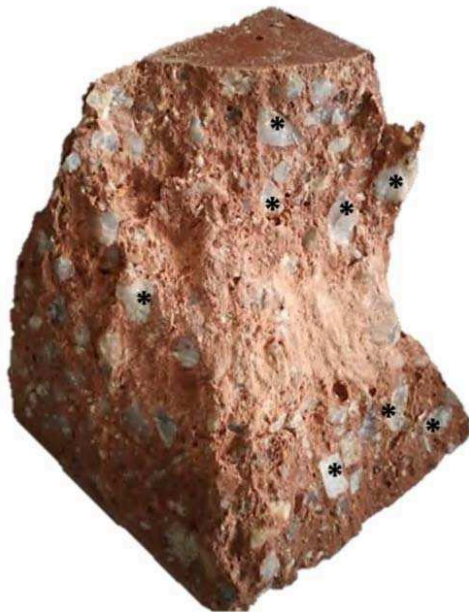
Figure 16. 100 x 100 x 100 mm geopolymer concrete prism after compressive strength breaking (Formulation GP14.5) with split aggregates (*).
