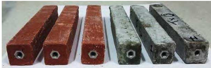
Figure 7. 2x2x16 cm geopolymer (left) and cement (right) mortar prisms showing stainless steel shrinkage bolts.
