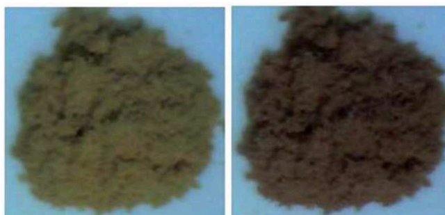
Figure 2.2: the characteristic color change of [\text{Fe}(\text{pz})\{\text{Ni}(\text{CN})_4\}] nanoparticles at high (left) and low (right) temperature
