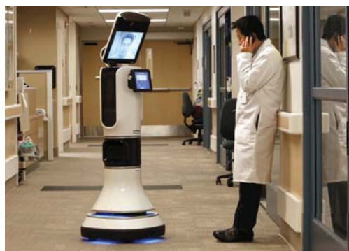
(d) RP-VITA : a medical robot that doctors can make remote visits to patients via PCs or iPads running the robots.
