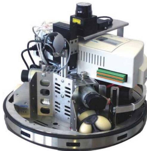
Figure 2.5: Robotino ® : a mobile robot system for education and research.
