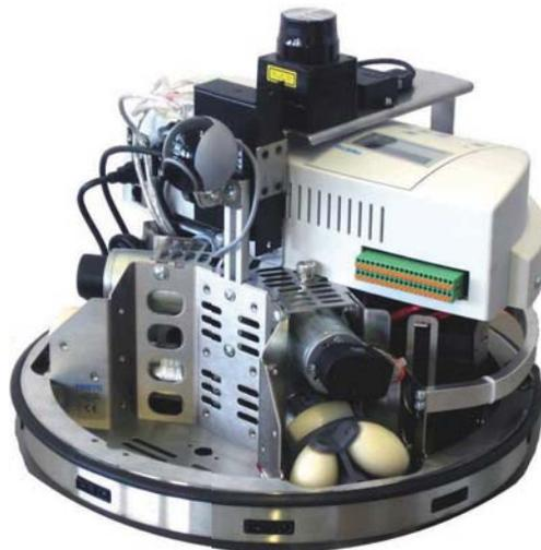
Figure 2.5: Robotino<sup>®</sup>: a mobile robot system for education and research.
