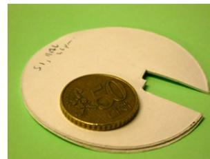
Fig. 12. THz tag : this paper is coded.
