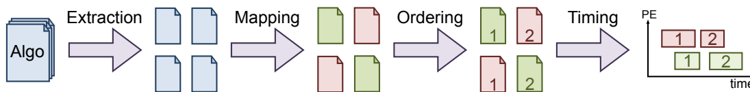
Figure 2.7 – Middle grain parallelism multicore scheduling on a two PEs (red and green) platform
