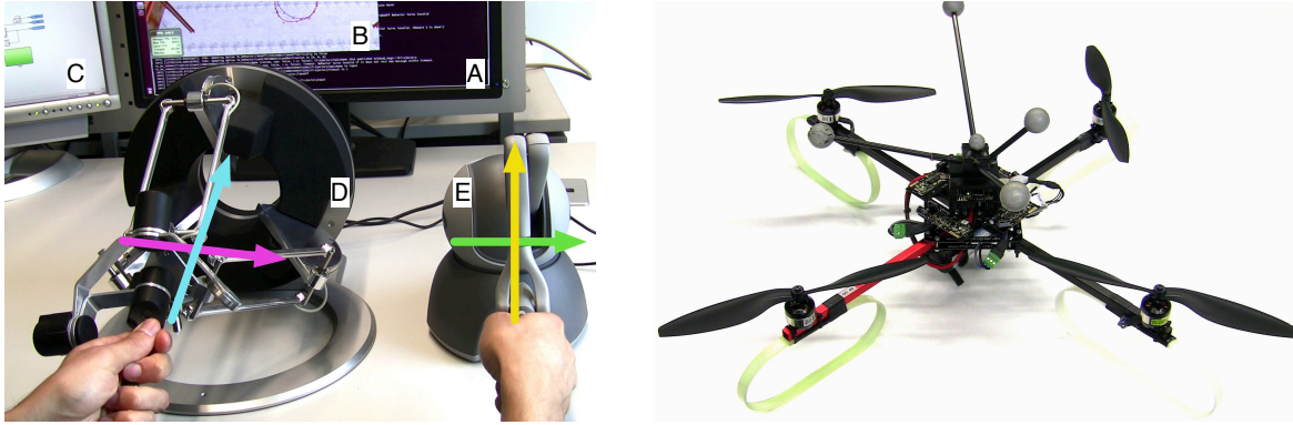
FIGURE V.14: Experimental setup. a) Software components of the framework and input devices: A) TeleKyb; B) SwarmSimX; C) Matlab; D) Omega.6, used to command changes of scale (magenta) and rotations (cyan); E) Phantom Omni, used to command translations along \vec{X}_W (yellow) and along \vec{Y}_W (green). b) The quadrotor used for the experiments.
