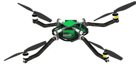
Fig. 26. CAD image of the new prototype with improved mechanics, actuation system, electronics, and an overall reduced mass and inertia.
