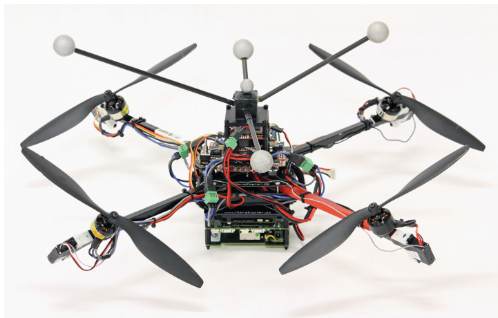
FIGURE VII.1: Picture of the holocopter prototype. The four propeller groups are slightly tilted. The red bar indicates the positive direction of the holocopter body axis
