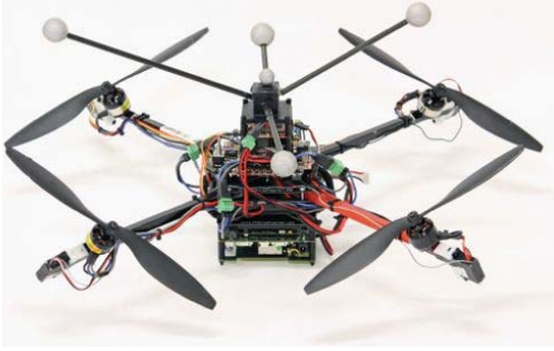
Fig. 1. Picture of the holocopter prototype. The four propeller groups are slightly tilted. Red bar: positive direction of the X_B holocopter body axis.
