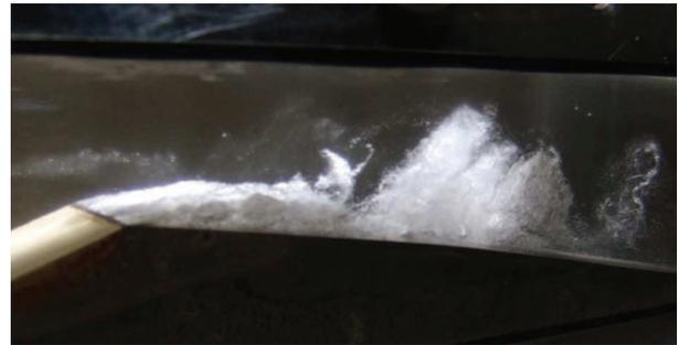
Figure 13. Photograph of the cavity, 8° Venturi.
