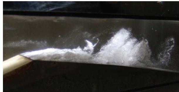
Figure 13. Photograph of the cavity, 8° Venturi.
