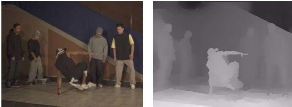
Figure 1.9 – A depth map with its associated texture frame. The higher the luminance value (brighter), the closer the object is to the camera.
