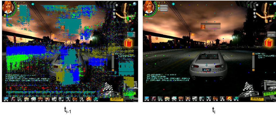
Figure 7.3 – Blocks having directions 7 (red), 8 (green), 9 (blue), 10 (cyan) or 11 (olive) as optimal Intra direction in two consecutive frames, sequence ChinaSpeed_1024 × 768 , QP 22.
