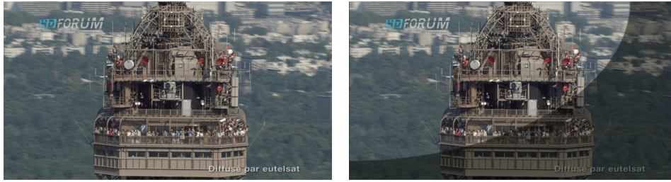
Figure 6.4 – Test sequence "Paris_fade" with fading effect: the illumination is gradually decreased as seen from left to right.
