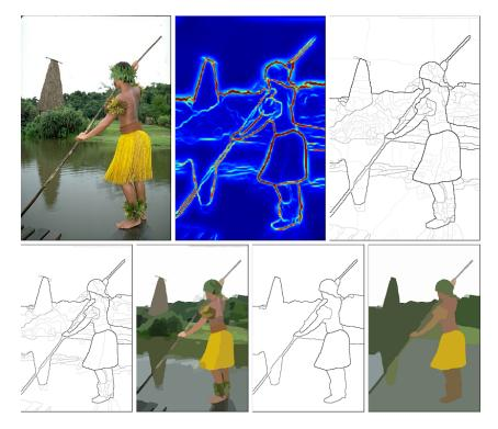
Figure 3.2: Hierarchical segmentation from contours [Arbelaez et al., 2011]. Top Left:Original image. Top Middle: Maximal response of contour detector gPb over orientations.Top Right: Weighted contours resulting from the Oriented Watershed Transform - Ultrametric Contour Map algorithm using gPb as input. Bottom: Contours and corresponding segmentations obtained by thresholding the UCM at levels 0.1(left), and 0.5 (right), with segments represented by their mean color.
