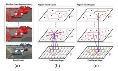
Figure 2.6: Multi-layer graph model [Kim et al., 2010b]. In (a), the graph nodes  $V^*$  consist of pixels V and regions  $V^{(l)}_{l=1,\dots,L}$ , generated by varying the parameters of the mean shift algorithm [Comaniciu and Meer, 2002]. An undirected edge  $E^*$  represents the relation between a pair of nodes. (b) and (c) show the examples of edges (violet lines) connected to one region and to one pixel, respectively.
