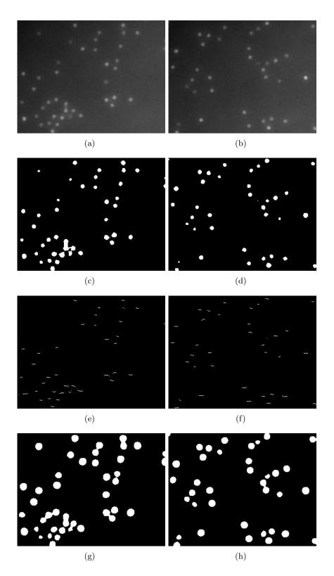
Figure 7.6: Visual comparison of different particle detection methods. (a, b) show two original video frames. (c, d), (e, f), (g, h) are the result obtained by the Otsu's threshold [Otsu, 1975], local maximum detection method, and wavelet based method [Padfield et al., 2011] respectively. 124
