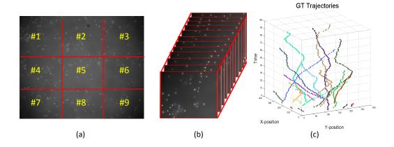
Figure 7.5: Illustration of ground-truth. (a) 9 subvideos (out of 16) extracted from the original large scale video; (b) Stack of frames in subvideo #1 annotated by human observers; (c) 3D visualization of a few trajectories tracked by observers in subvideo #1.
