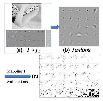
Figure 2.5: (a) Polka-dot image is convolved with a bank of filters. (b) Textons found via K-means with K = 25, sorted in decreasing order by norm. (c) Mapping of pixels to the texton channels. The dominant structures captured by the textons are translated versions of the dark spots. [Malik et al., 2001].
