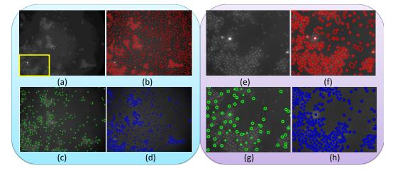
Figure 7.2: Illustration of active colloid detection. In light-blue block: (a) a video frame with highly dense colloids; (b) result segmented only by level set [Li et al., 2008]; (c) result detected with Gaussian smoothing and circular Hough transform; and (d) result obtained by the combination of level set and circular Hough transform. In light-purple block: (e) zoom in version of the yellow rectangle shown in (a); and (f-h) are the zoom-in results corresponding to (b-d) respectively.
