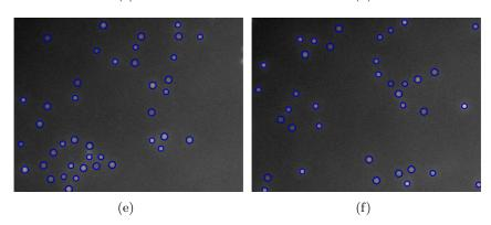
Figure 7.7: Visual comparison of different particle detection methods. (a, b) show two original video frames. (c, d), (e, f) are the result obtained by the method proposed in [Sbalzarini and Koumoutsakos, 2005] and our method respectively.
