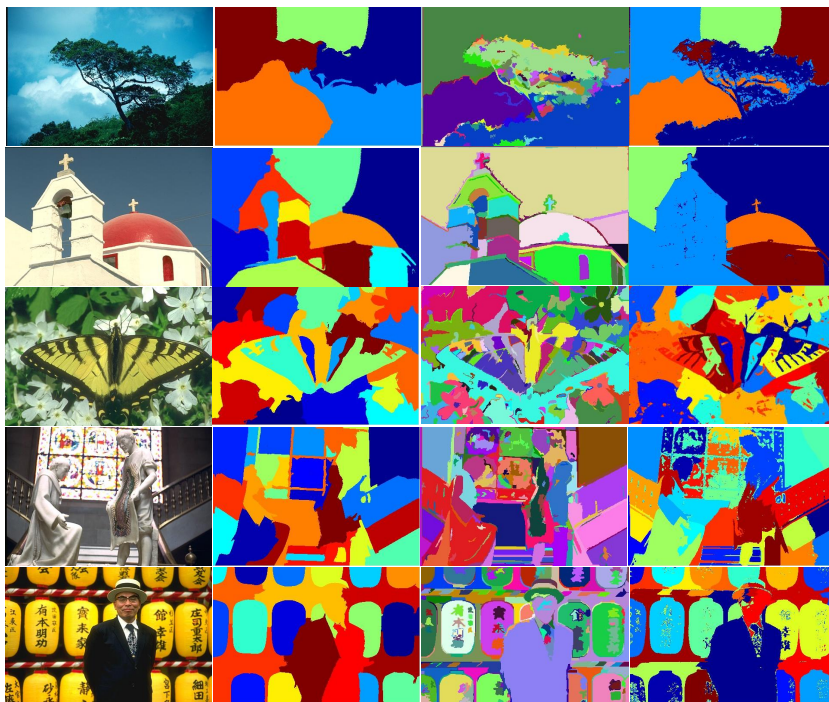
Figure 5.4: Visual comparison of our results with other methods on the Berkeley database (examples presented in column-wise, from left to right, are respectively the original images, NCut, GBIS and our results).
