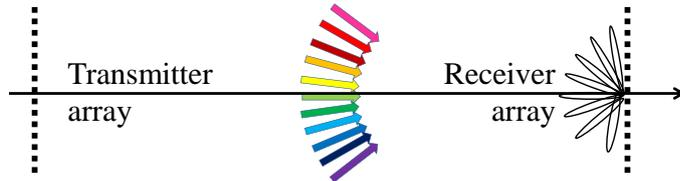
Fig. 5.4.2 DFT-SM for aligned linear arrays
