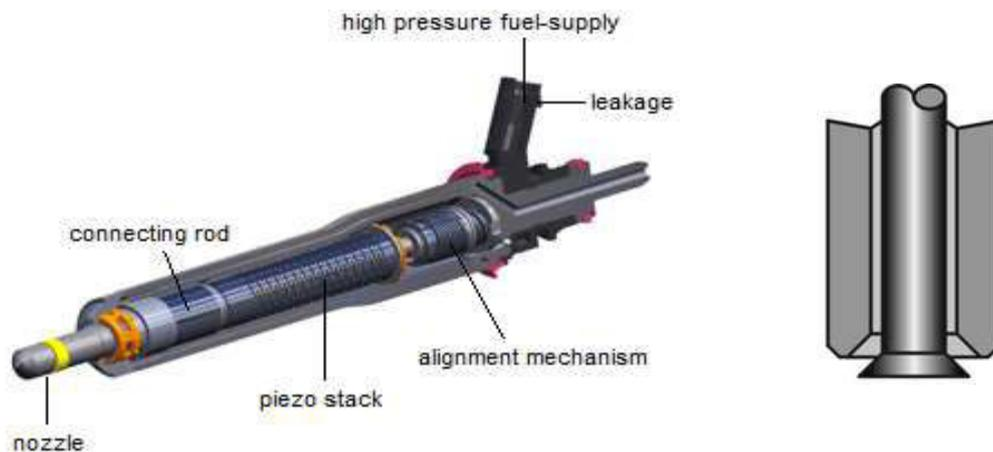
Figure 2-4: Schematics of a directly-actuated piezo-electric outward-opening injector [3] (left) and of an outwardly opening nozzle [1].
