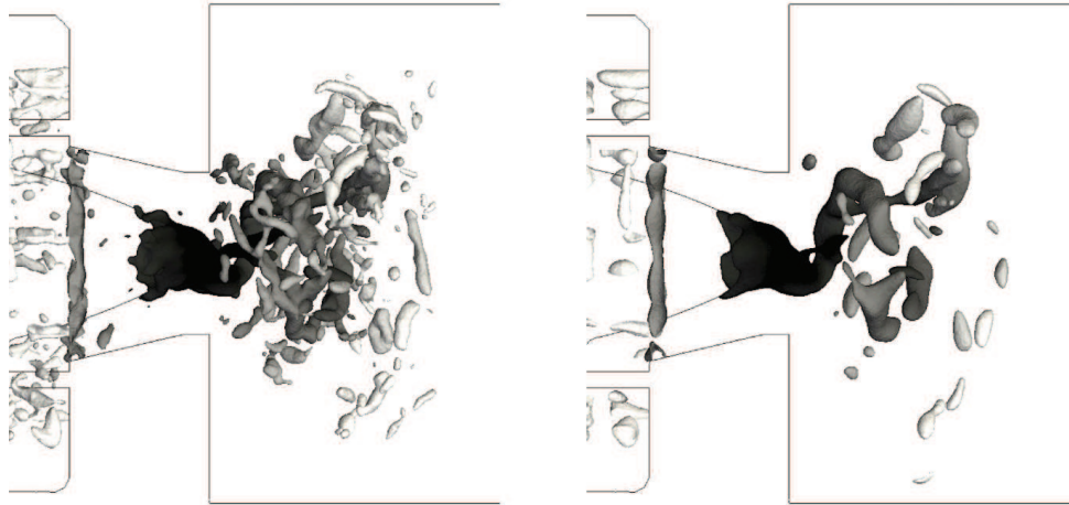
FIG. 27. Extraction of the PVC with Gaussian filter (left) and 8th order filter (right), on the 878M mesh.
