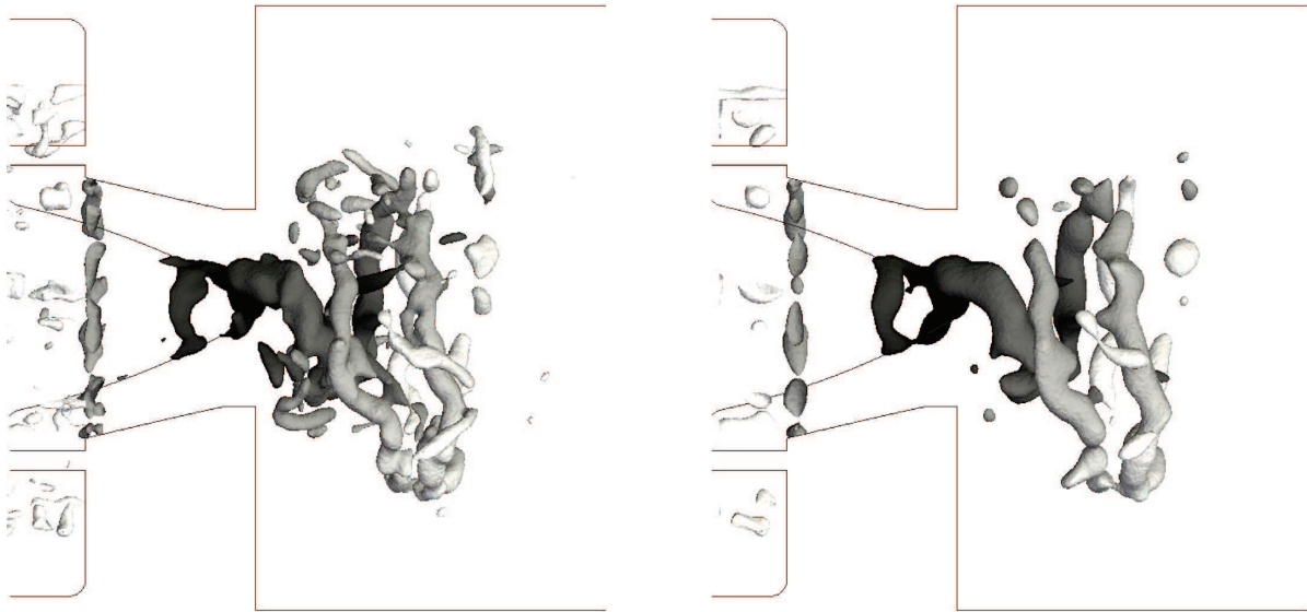
FIGURE 4.32 – Extraction of the PVC with Gaussian filter (left) and 12th order filter (right), on the 110M mesh
