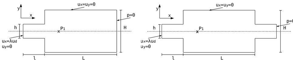
Figure 4: Channels with prescribed velocity profile  $\mathbf{u}_d$  on the inlet, no-slip wall law and null pressure on outlet. Left :  $h = 10, H = 3h, l = 3h, L = 30h$ . Right :  $h = 10, H = 30, l = l_{in} = l_{out} = 3h, L = 8h$ . A velocity probe is placed near to the expansion on the symmetric axis.
