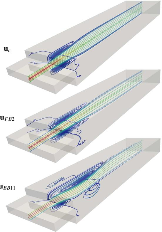
(c) Streamlines for three-dimensional steady flows,  $A_i = 8$ .
