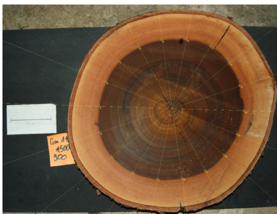
Calculation of heartwood, sapwood and bark area using Image processing. The image shows position of 18 radii
