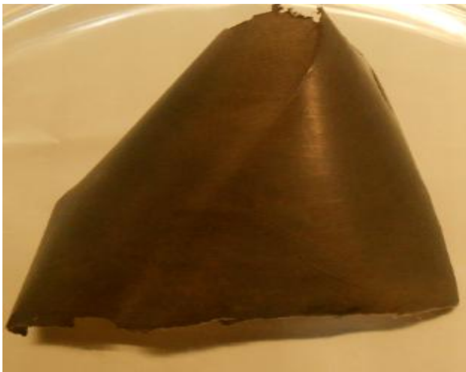
Figure 53 : Film du nanobiocomposite PLA/PLAgMA/1OG
