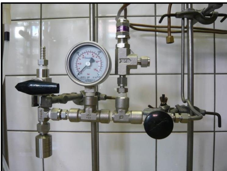
**Figure 8.2:** Metallic minireactor (10 mL) for high pressure (5 MPa) copolymerizations
