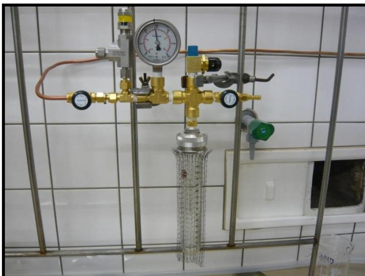
**Figure 8.1:** Fisher-Porter bottle (100 mL) used for copolymerizations up to 1 MPa of  $\text{CO}_2$
