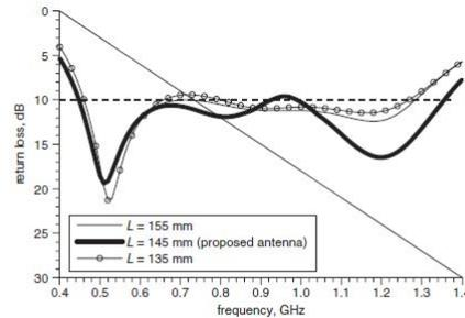
Fig. 3 Measured return loss against frequency for different length of fork-like monopole antenna
