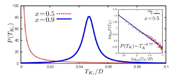
Figure 8.9: Distribution of Kondo temperatures  $P(T_{K_i})$  (calculated from Eq. 8.8) in the weak coupling case  $(J_K = D)$  for x = 0.5 (red dashed line) and x = 0.9 (blue solid line). Other parameters are  $n_c = 0.5$  and Z = 5. The power-law behavior of the x = 0.5 is an evidence of a Non-Fermi Liquid behavior that is expected when  $x \approx n_c$ . Inset: Double-logarithm plot of  $P(T_{K_i})$  for x = 0.5. The obtained power-law exponent is -0.77.
