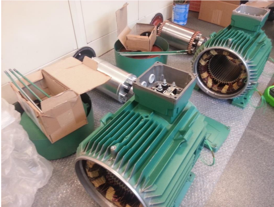
Fig.3. 21 Two commercial IMs dismantling for the following prototyping
