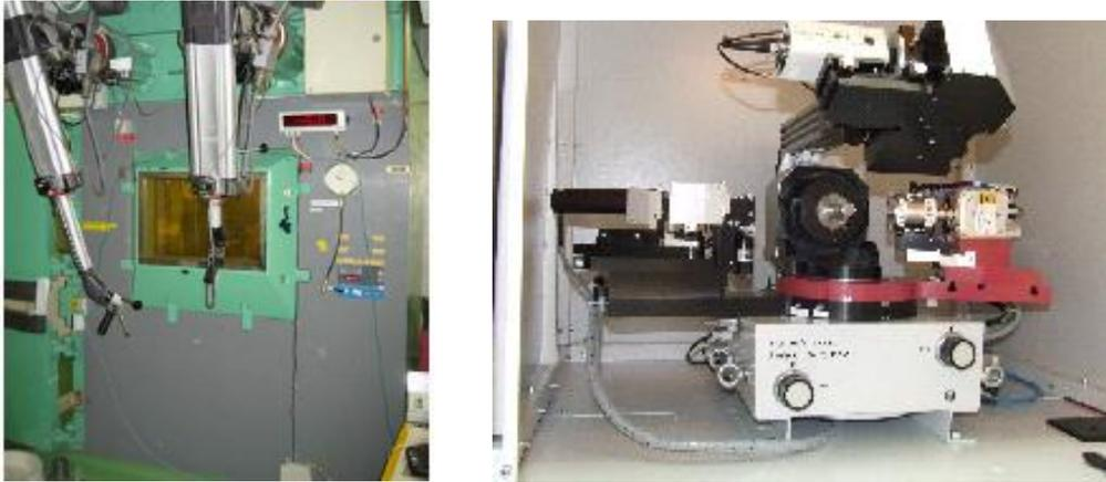
Figure 126: Hot cell where the XRD equipment is placed (left) and the equipment itself (right)
