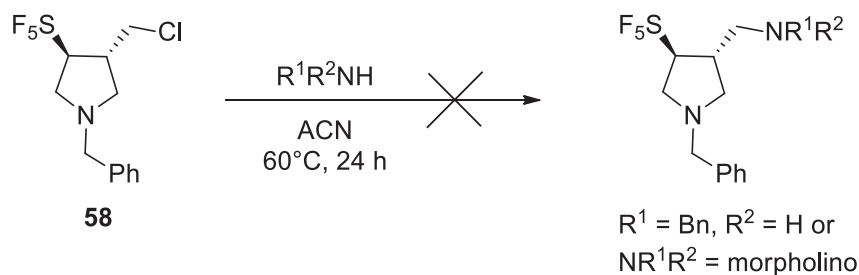
Scheme 87: Attempts for the nucleophilic substitution of chloride 58 with benzylamine or morpholine.
