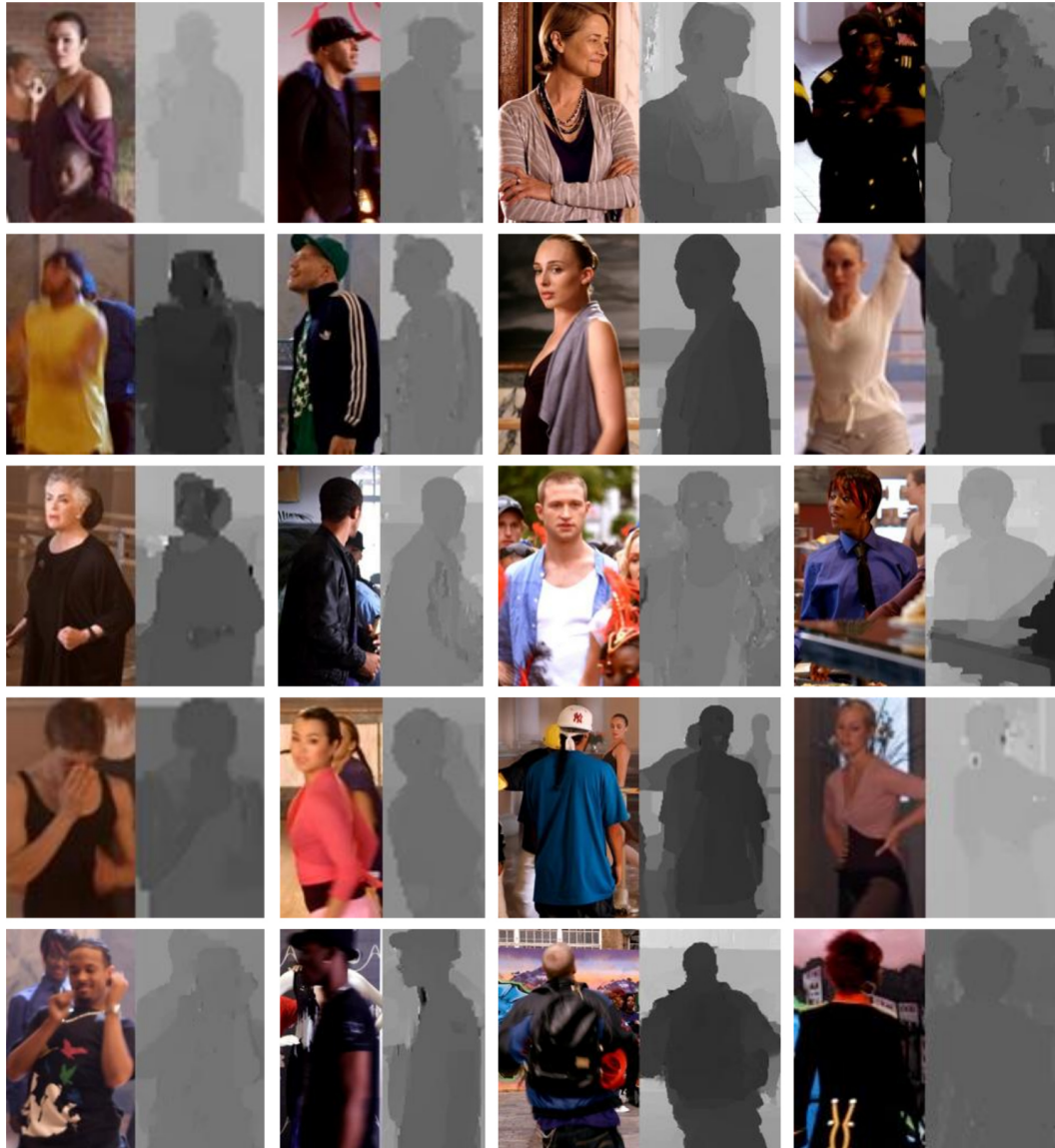
Fig. 4.21: Examples of automatically harvested person examples. We show side-by-side the cropped image and the cropped disparity map of each example. These examples were collected from stereoscopic movies. They were associated to a highly confident score by the joint HOGcomb detector, and a low score by the appearance-based HOG detector.
