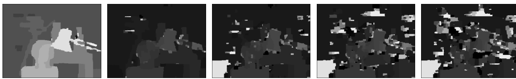
Fig. 4.5: Disparity maps from a rectified image pair (left) and unrectified image pairs with 1 to 4 pixels of vertical miss-alignment (four images on the right).
