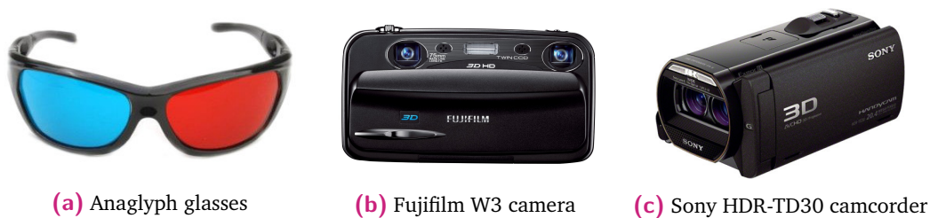
Fig. 1.5: Examples of devices for 3D movies: anaglyph glasses (a) allow watching 3D movies screened using the anaglyph technique. Consumer-level cameras (b) and camcorders (c) are available to capture stereoscopic stills and videos.
