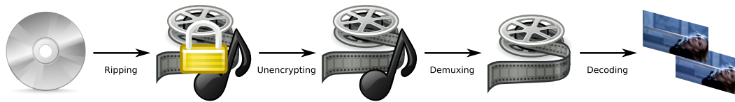
Fig. 4.1: Pipeline used to extract stereo pairs from 3D Blu Ray disks. The first three steps, from Ripping to Demuxing, are handled by the MakeMKV software ( http://www.makemkv.com/ ). The decoding is performed by a modified version of a reference MPEG4 decoder.
