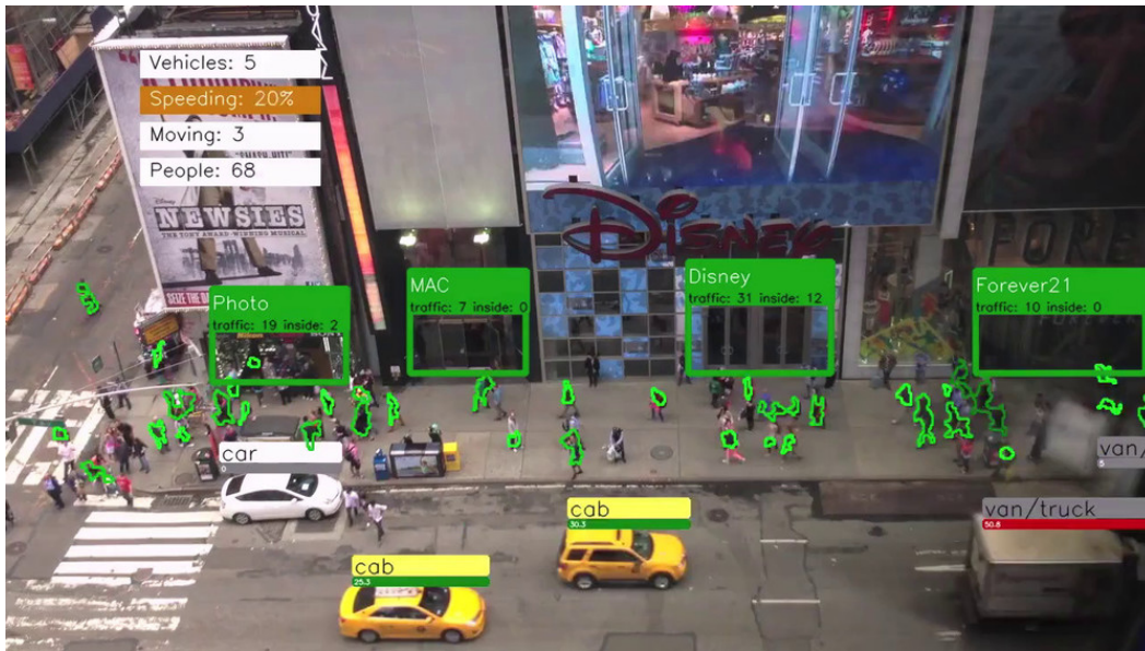
Fig. 1.1: Example of surveillance system output a : the system detects and tracks each person and vehicle in its view. It monitors the speed of the vehicles to detect speeding ones. It also keeps tracks of persons going in and out of each store.
