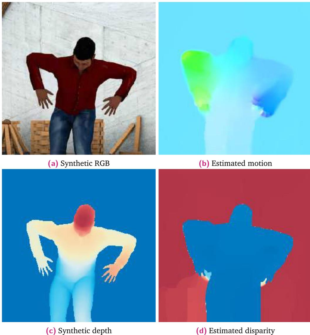
**Fig. 7.1:** Example of synthesized upper body pose example. Stereoscopic pairs of sequences of synthetic RGB frames (a) are generated using Blender, as well as a sequence of depth ground truth (c). Motion (b) is estimated from one frame of the left view to the next, while disparity (d) is estimated from a stereoscopic pair.
