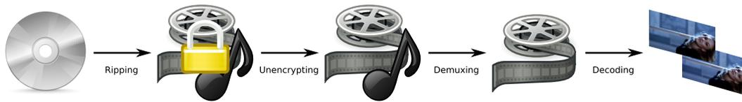
**Fig. 4.1:** Pipeline used to extract stereo pairs from 3D Blu Ray disks. The first three steps, from Ripping to Demuxing, are handled by the MakeMKV software (<http://www.makemkv.com/>). The decoding is performed by a modified version of a reference MPEG4 decoder.
