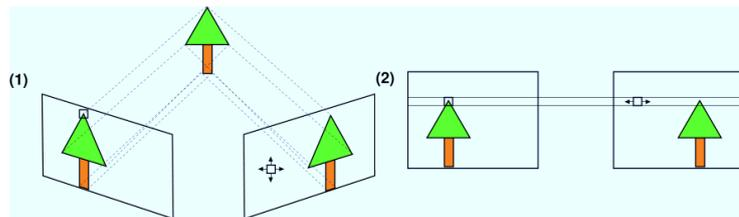
**Fig. 4.4:** Rectification makes epipolar lines coincide in stereo pairs<sup>5</sup>.
