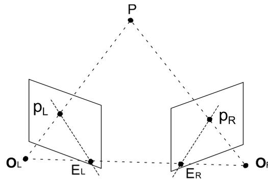
**Fig. 4.3:** Epipolar geometry<sup>4</sup>.
