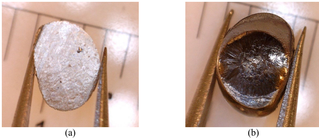
Figure 21: Sample OUZr_7 before and after a laser pulse sequence. In figure (b) the circular trace of laser spot can be clearly seen
