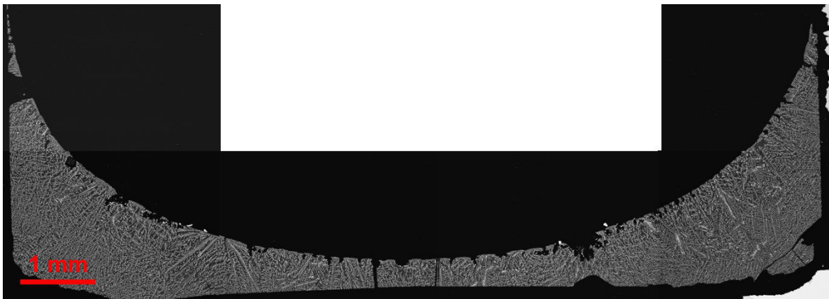
Figure 1: Back-scattering electrons (BSE) image of the cross section of the solidified sample CORIUM_1
