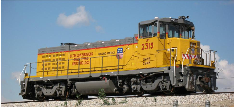
Figure 1.5: The Railpower Green Goat locomotive.
