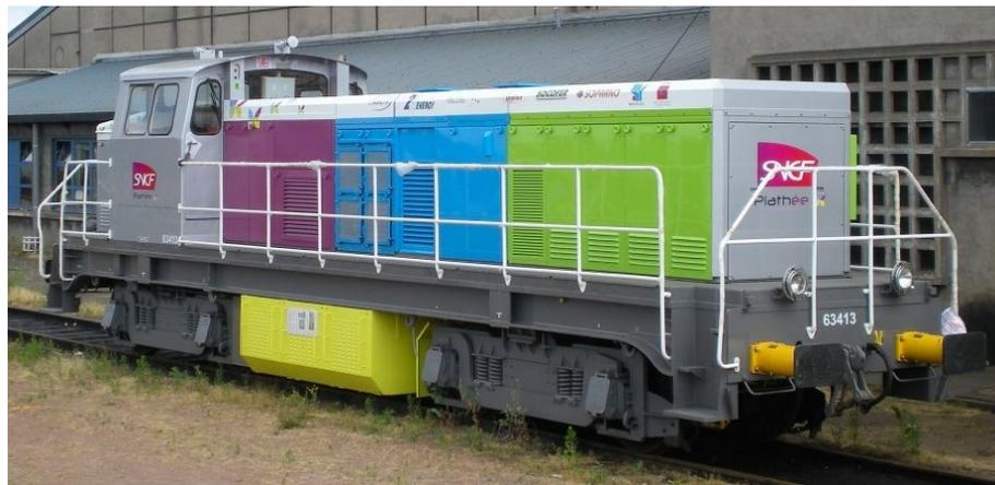
Figure 1.7: SNCF Hybrid Electric Locomotive - Plathee project.
