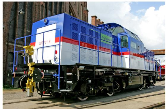
Figure 2.6: Freight Hybrid Electric locomotive
