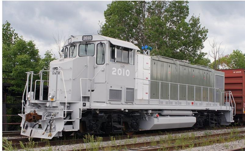
Figure 1.6: Fuel cell-hybrid switcher platform vehicle.
