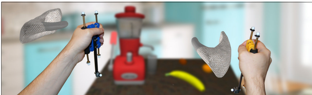
Figure 6.1 – Grasping virtual objects in a bimanual scenario with the Virtual Mitten. Each hand holds an elastic device to control a corresponding mitten. The grip force applied by the user is measured to grasp virtual objects and to generate pseudo-haptic feedback.
