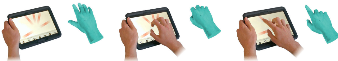
Figure 3.1 – Controlling the posture of a hand model with THING. Our approach is based on a morphologically-consistent multi-touch interface that applies the real motion of the user on the virtual model. For example, performing a grasping gesture or a pointing gesture replicates it on the hand model.
