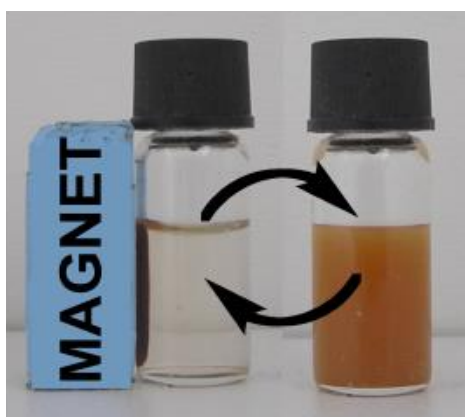
Figure 1. Picture illustrating the concentration of MNPs under the influence of a magnet (MNPs come close to the vial wall), and the dispersion of MNPs upon the field removal.
