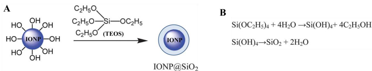
Scheme I-5. (A) Formation of silica coated IONPs (core-shell) through hydrolysis and condensation of TEOS. (B) Hydrolysis and condensation of TEOS.
