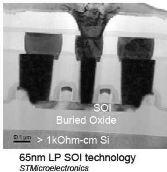
FIGURE 1.28: SEM 65 nm SOI CMOS de ST Microelectronics [38]
