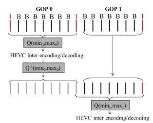
Figure 3.2: The process used for the GOP-wise method. This method keeps the temporal coherence inside a GOP and between two GOPs to better exploit temporal predictions. The quantization and inverse quantization steps are referred to as Q and  $Q^{-1}$  respectively, and  $min_i$  and  $max_i$  are the minimum and maximum values in the GOP i.
