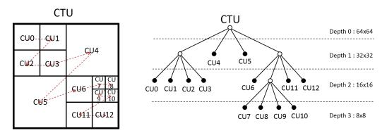
Figure 2.3: Illustration of the HEVC CU quad-tree partitioning. The CUs are processed in the Z-scanning order shown by the red arrows.
