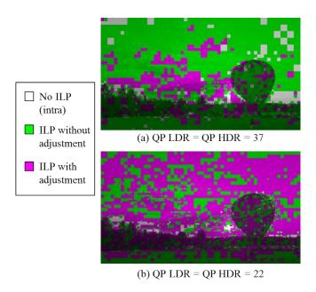
Figure 4.8: Mode usage for our template based ILP with extended templates and adjustment factor.
