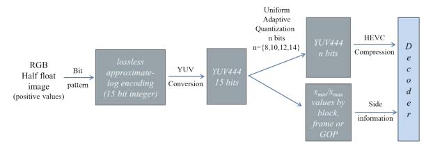
Figure 3.1: Adaptive Uniform Quantization scheme for floating point HDR image encoding.
