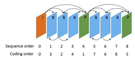
Figure 2.7: Example of GOP structure. In this example, a B frame may be used for the prediction of other B frames. This is called a hierarchical GOP structure.
