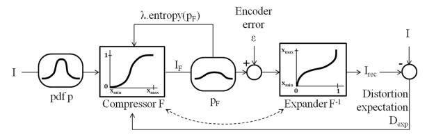
Figure 3.6: Statistical model of the HDR compression scheme.
