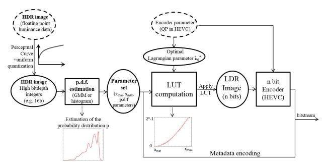
Figure 3.7: Overview of the HDR compression scheme based on the Rate Distortion optimized tone mapping.
