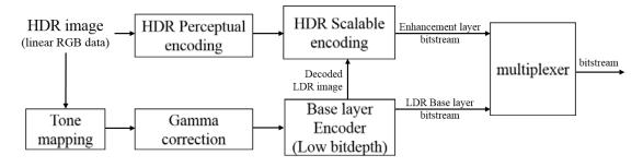
Figure 2.15: HDR Scalable encoding scheme.
