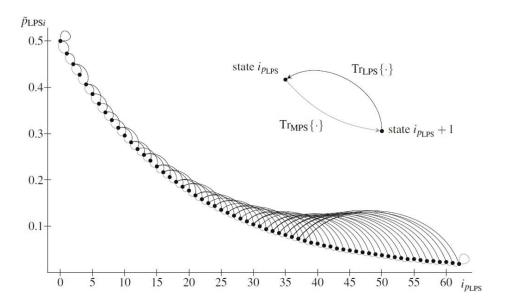
Figure 2.10: CABAC states update.  $\tilde{p}_{LPS_i}$  is the probability of the least probable symbol (LPS) at a given state of the CABAC context. It decreases according to the arrow  $Tr_{MPS}$  when a most probable symbol (MPS) is encoded. Conversely, when the least probable symbol is encoded,  $\tilde{p}_{LPS_i}$  increases according to  $Tr_{LPS}$ .
