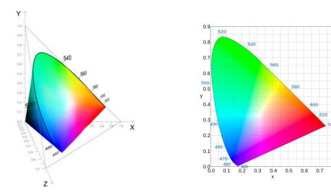
Figure 1.4: Left: 3D representation of the CIE 1931 XYZ colorspace. Right: CIE 1931 xy chromaticity diagram.
