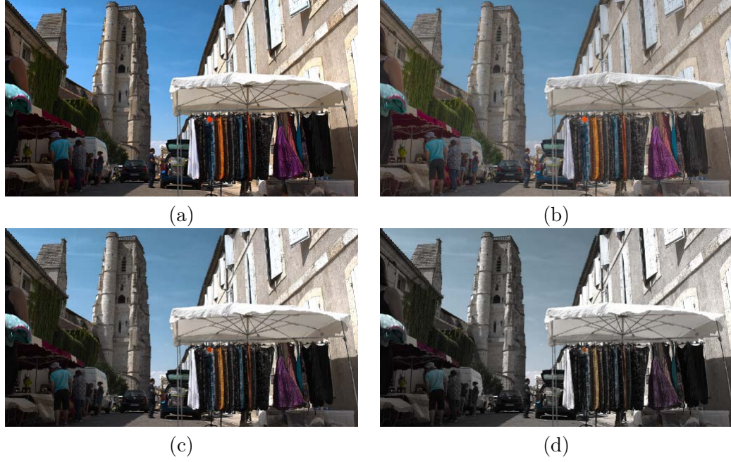
Figure 5.3: u'v' prediction results on a frame of the Market3 sequence. (a) Original HDR image. (b) Tone mapped image with the TMO in [85] using s = 0.6 and \gamma = 2.2 . (c) HDR color prediction from [62] (i.e. assuming s = 1 and \gamma = 2.2 ). (d) HDR color prediction from [68] (i.e. assuming \frac{\gamma}{s} = 1 ).
