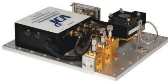
FIGURE 2.9: Example of a frequency multiplier chain LO from VDI (Picture from Hesler et al. [25])
